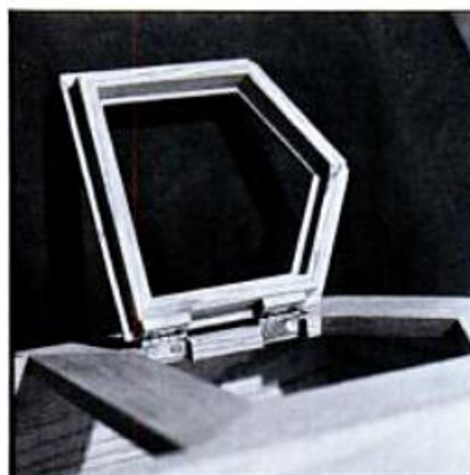
Small glueblocks in the door enable butt hinges to be used on an overlay door.
