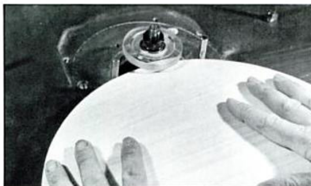
One way to shape outside curves is to guide the edge against two pins. This method will work only with circular shapes. A plexiglass disk serves as a guard.
