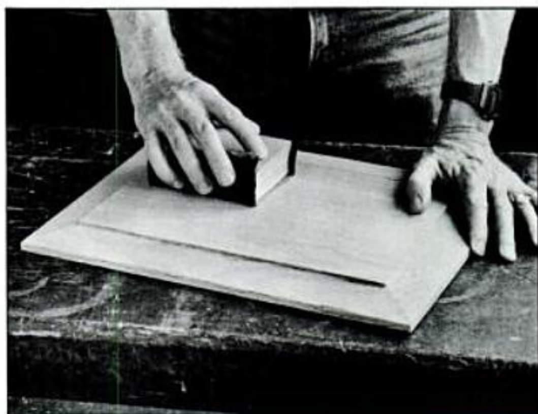
A sealer coat of dilute shellac locks the wood fibers in place. A light scuff sanding with fine sandpaper cuts the fibers off smoothly.
