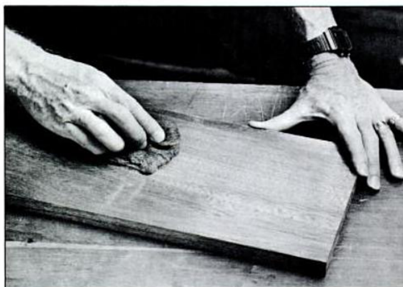
Rubbing with 0000 steel wool will give a rubbed satin look. Switch to pumice with water or oil for greater gloss. For maximum gloss, finish up with rottenstone.
