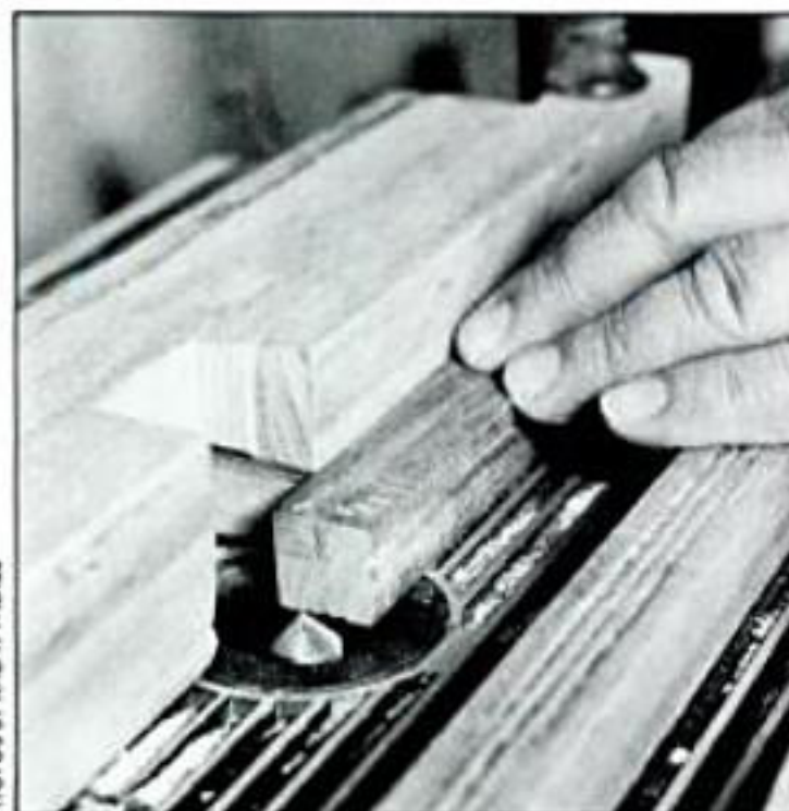
Cut the decorative grooves with a V-grooving bit.
