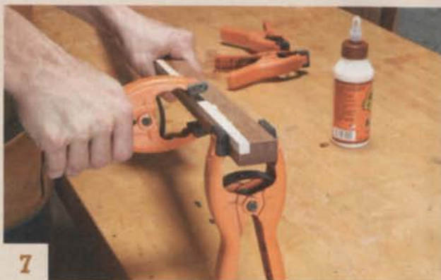
7 Create the decorative edging by gluing a large piece of stringing into a rabbet cut on the inside edge.
