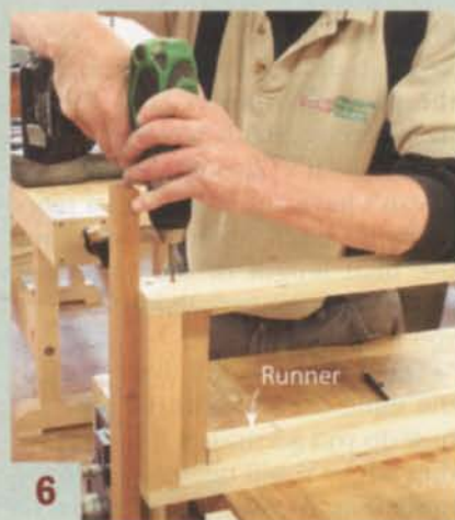
6 Assemble the carriage that holds the runners.
