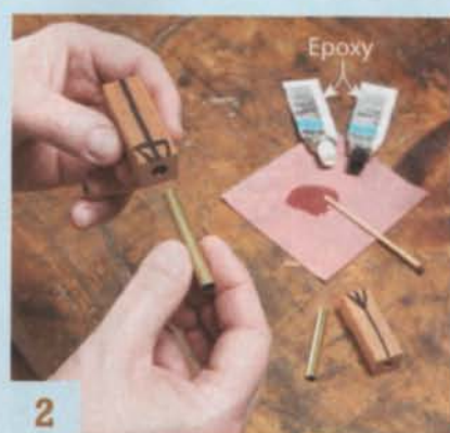
2 Start by gluing the brass tubes from a pen kit into a pair of wood pen blanks. Mark the blanks to keep the grain oriented correctly.
