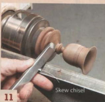
11 Embellish the stem with thin diameters and delicate details.
