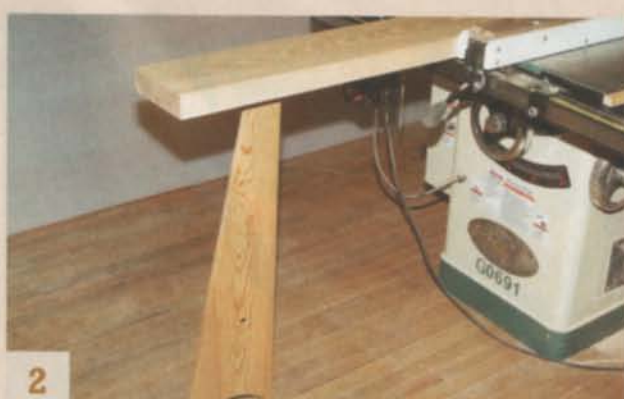
2 Use a support to keep the blank's leading edge flat on the saw table, so you can precisely position the fence and the blade between cuts as you rough out the profile.
