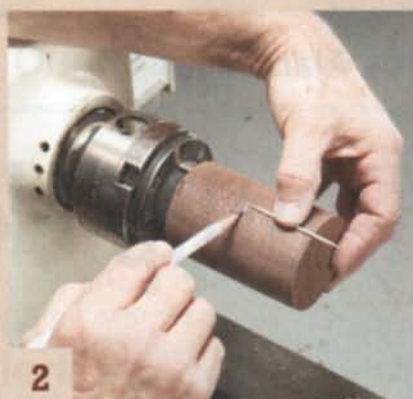
2 Use a toothpick to set the depth of the hollow cup. Mark the line all the way around the blank.
