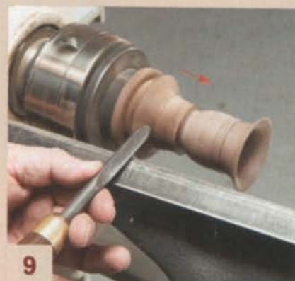
9 Shape the base and begin to reduce the stem's diameter with the detail/spindle gouge. Work from large to small diameters.
