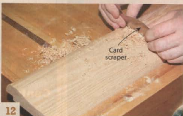
12 Complete the molding by smoothing the contoured surface with a card scraper or sandpaper wrapped around a can, plastic pipe or mailing tube.
