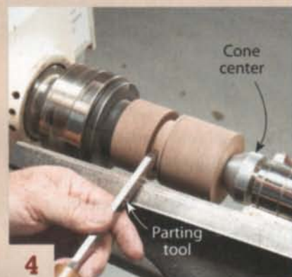
4 Establish the bottom of the cup by cutting in slightly below the line marked earlier. Support the blank with a cone center.
