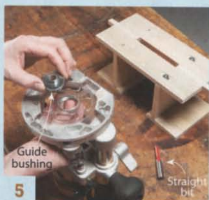
5 Install a guide bushing in your router to ride in the slot in the top of the jig. Use a straight bit for routing.
