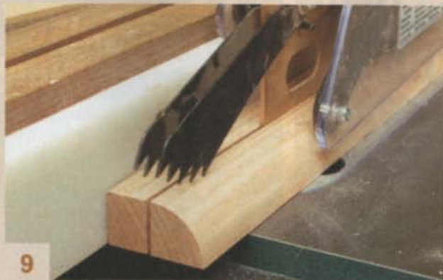
9 Cut the quarter-round molding from a wide blank that has been rounded over.
