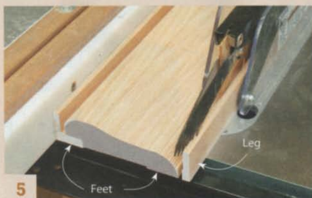
5 Saw off the legs with the blank facing right-side up. Feet created by routing the shallow dado support the blank.
