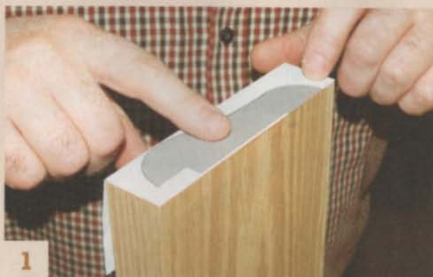
1 Attach the top section of the pattern to a large rectangular blank. Make sure the pattern is parallel with the bottom edge.
