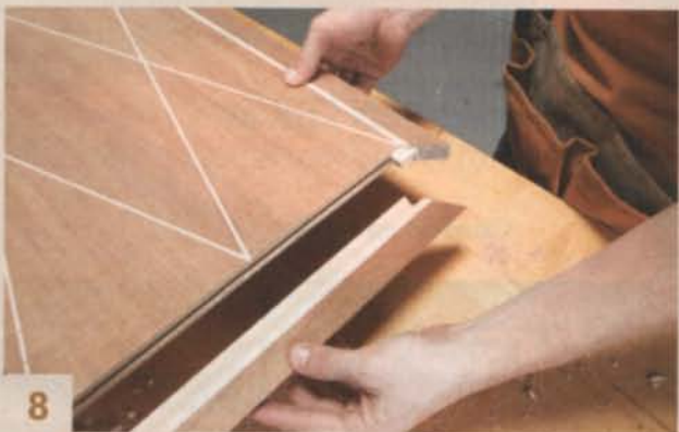
8 Install the edging, using splines to level the pieces with the surface of the veneered top.
