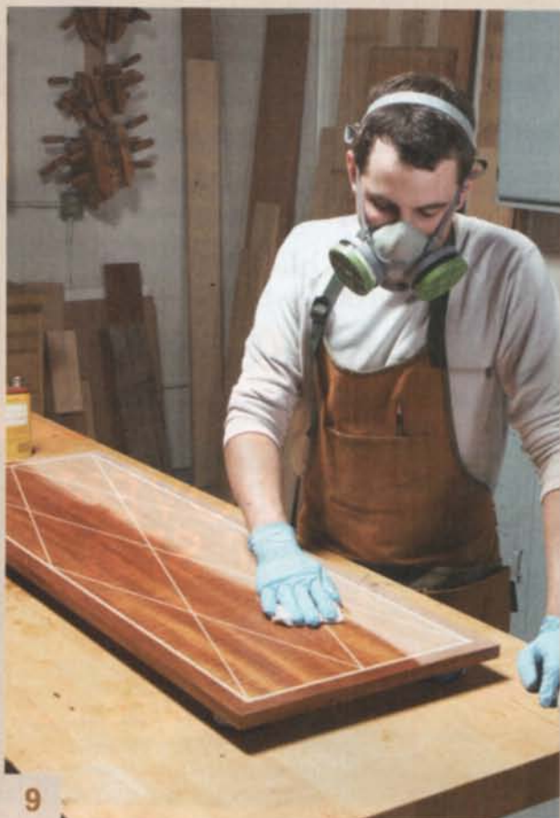
9 Apply a finish. I prefer to wipe on tung oil, followed by polyurethane.
