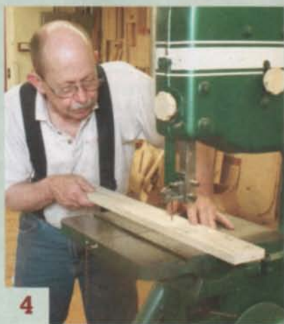
4 Saw the arc, staying close to the line. Make another piece just like this one. They will become the jig's runners—the curved parts that guide the router.
