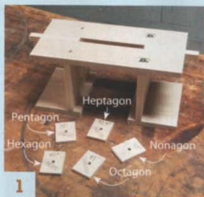
1 Index blocks with lines drawn at different angles allow using the jig to create pens with a variety of geometric shapes.
