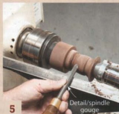
5 Use a detail/spindle gouge to roughly shape the outside of the cup, including the flared rim.
