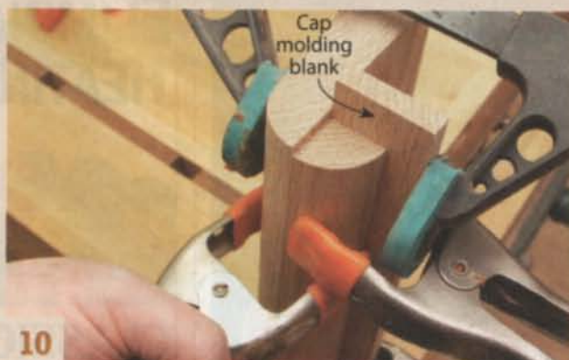
10 Use the blank for the cap molding as a temporary stop to align the quarter-round molding and the top molding for gluing.
