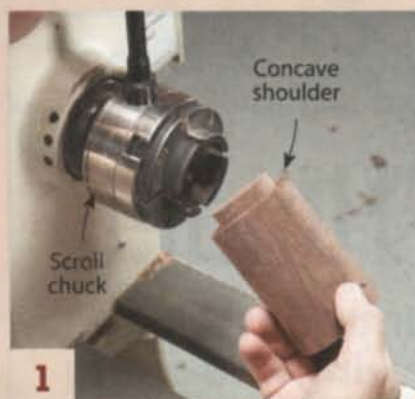
1 Mount the blank in a scroll chuck after turning a tenon on one end. The tenon's shoulder must be slightly concave.
