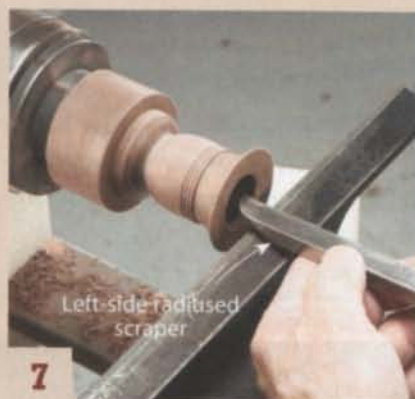
7 Hollow the cup with a radiused or round-nose scraper. Insert the tool without touching and engage the near side as you draw it out.
