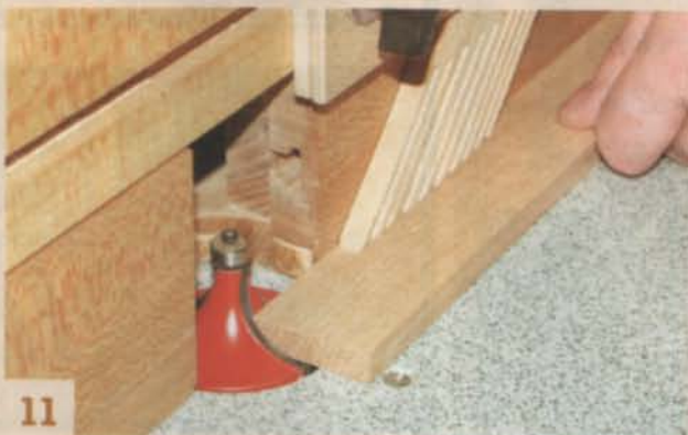
11 Create the cap molding's profile by using a portion of the roundover bit. Lower the bit slightly below the table and position the fence in front of the bearing.
