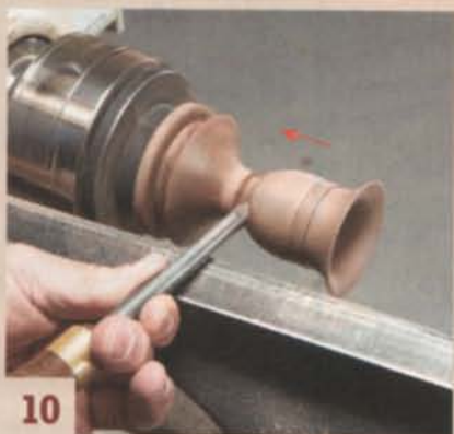
10 Shape the bottom of the cup and its transition to the stem by working in the opposite direction.
