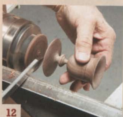
12 Part off the completed holder with a parting tool or the skew and a light touch to grasp the holder as it separates.
