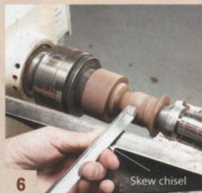
6 Refine the bowl's shape and add decorative elements such as tiny beads with the gouge and the skew chisel.
