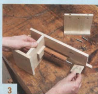
3 Disassemble the jig to install the blanks and the index block. Then reinstall the right leg assembly and tighten the wing nut.
