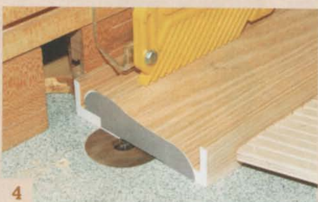
4 Rout a shallow dado on the bottom of the blank. Install featherboards to hold the blank against the fence and flat on the table.
