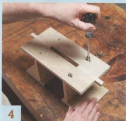
4 Lock everything in place by screwing the stove bolts into the cross dowels that are mounted in the right leg assembly.
