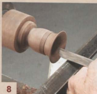
8 Clean the hollowed surface by shear scraping. Raise the scraper onto a corner at 45°. Then work the near side, as before.
