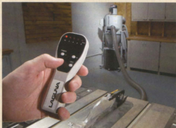
A remote control —standard equipment on some models—enables you to turn the cyclone on or off from wherever you're working.
