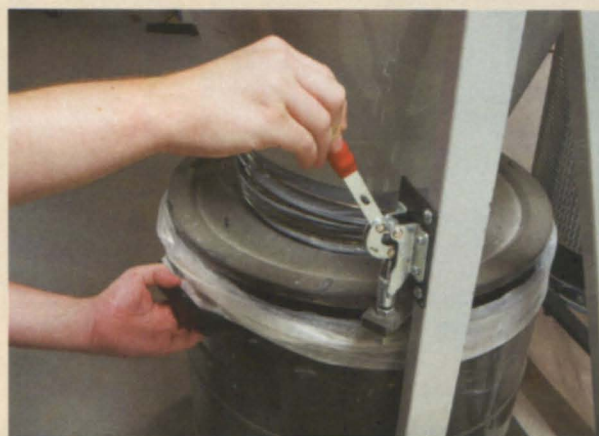
Toggle clamps for detaching the barrel from the cyclone make it much easier to take out the trash.
