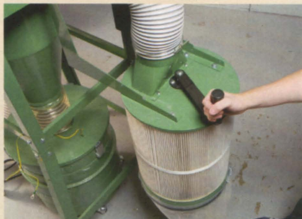
A mechanical agitator knocks dust off the inside of the filter. Keeping the filter clean maximizes airflow.
