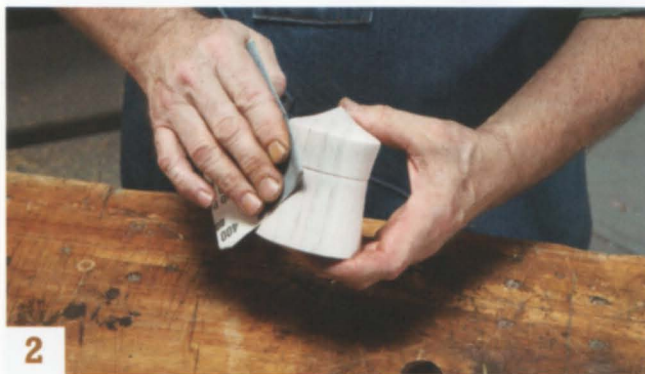
2 Sand lightly to ghost back the walnut color. Then apply lacquer, wax or a clear water-based finish.
