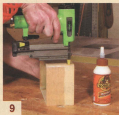
9 Nail the drawers. The sides are rabbeted into the front and back pieces.
