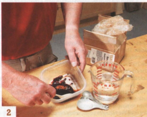
2 Make tannic acid for the second solution. Mix dry powdered tannin with a small amount of water to make a paste, then add more water.
