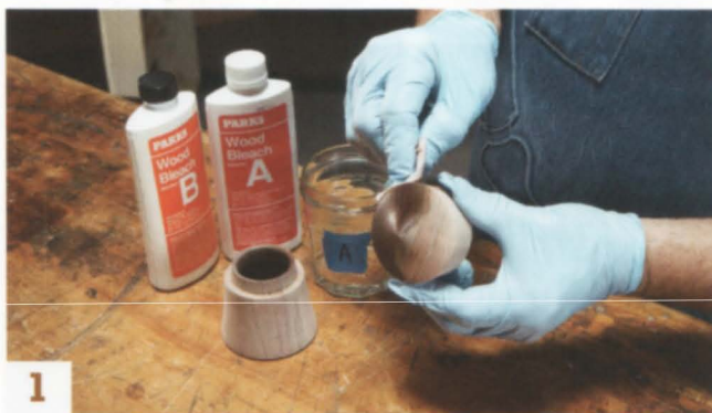
1 Remove the wood's natural color with two-part wood bleach. Several applications may be necessary.
