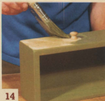
14 Paint over the texturing compound after the compound dries.
