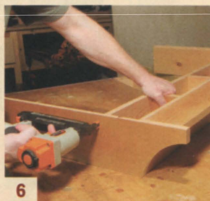
6 Fasten the sides. They're joined to the shelves with biscuits, too.
