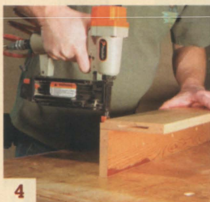
4 Fasten the bottom shelf to the peg board.
