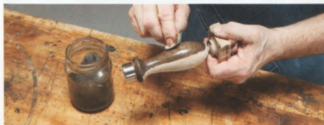
Wiping a solution created by immersing steel wool in household vinegar onto woods that contain high amounts of tannic acid causes a chemical reaction that turns the wood black.
