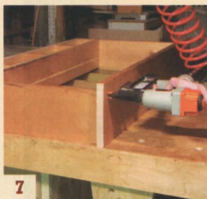
7 Add the top. Using a nail gun makes assembly go fast.
