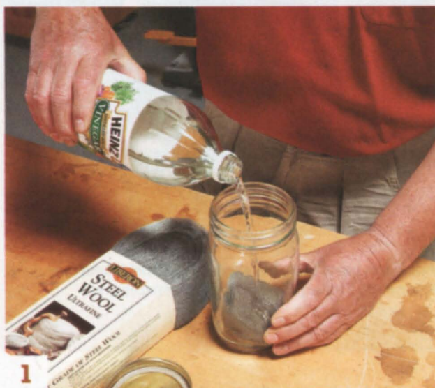
1 Dissolve steel wool in vinegar to make the first of two solutions you'll need. The pad should completely dissolve in about one week.
