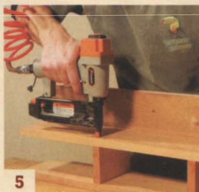
5 Fasten this assembly to the drawer dividers and middle shelf, using biscuits and nails.
