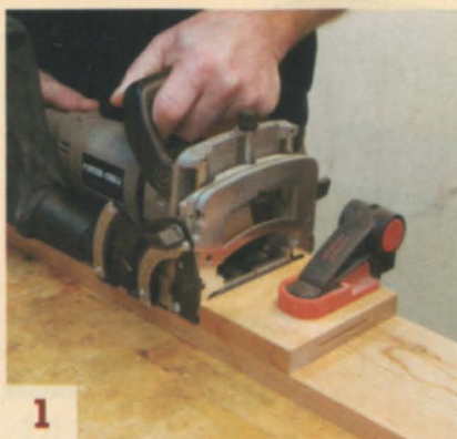
1 Cut biscuit joints in the drawer dividers.
