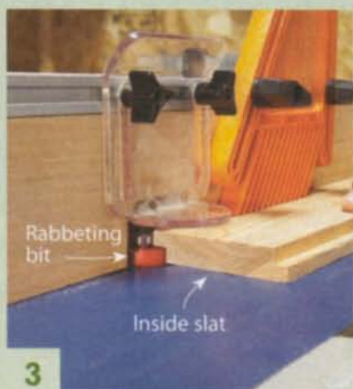
3 Rout rabbets on both edges of the inside slats, but on opposite faces, so the ends look like a "Z." The end slats are rabbeted on only one edge.
