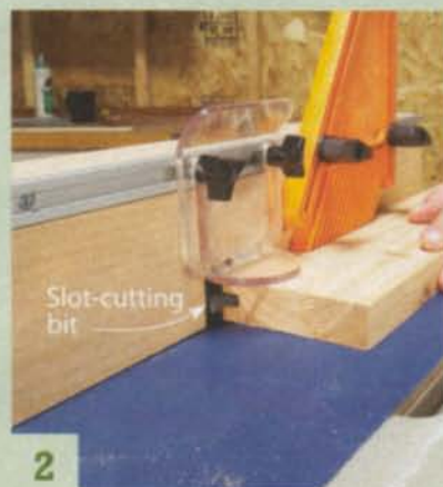
2 Rout a centered groove in one edge of each rail, to house the slats.
