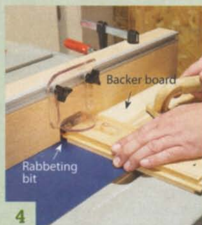
4 Rout tenons on the ends of each slat, using a rabbeting bit. Make one pass on each face. Use a backer board to guide the workpiece and prevent blowout.
