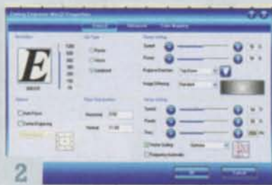
2 The Epilog's settings are adjusted in a printer driver window on your computer. By adjusting rate, frequency, intensity and other parameters, a variety of materials can be engraved or cut.
