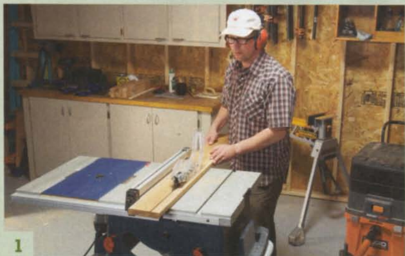
1 Start by ripping the rails to width from 5/4 cedar boards. This project is made with materials from the home center.
