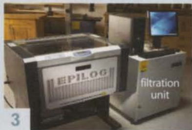
3 The laser beam produces smoke and fumes, so you'll also need an external exhaust system or a portable filtration unit.
