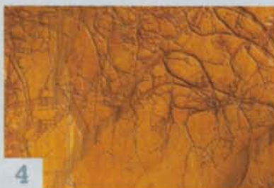
4 The future for CNC laser woodworking is wide open. This shallow relief carving, based on a photo of a tree, cuts through one layer of plywood to reveal the layer below. It's a beautiful effect that we found with creative experimentation.
