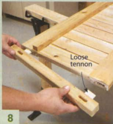
Glue and clamp the legs to the side panels. Swab glue in the mortises and on the ends of each panel. Install the BeadLOCK tenons; then install the legs.
