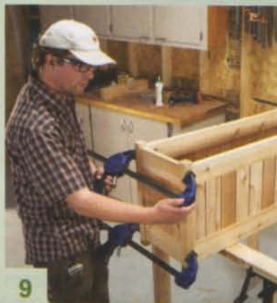
Complete the planter by gluing the end panels between the assembled sides.
