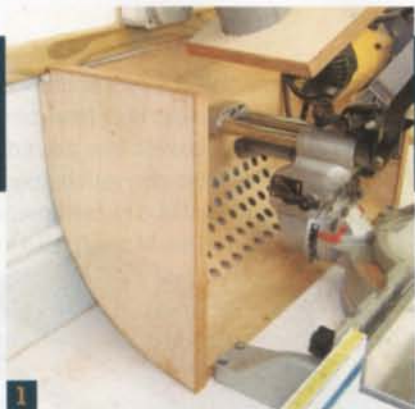
1 A curved front with air holes is the heart of my collection box. The wall behind the saw and the bench that it sits on act as the back and the bottom of the box.
