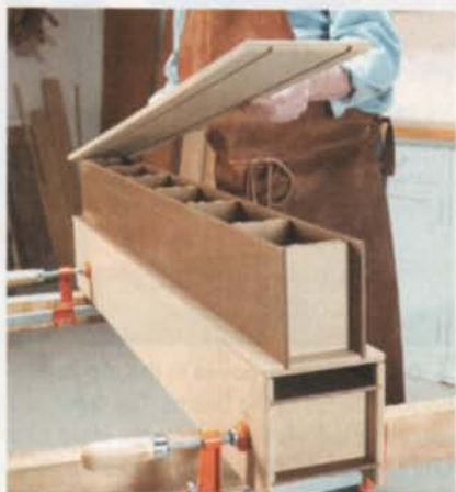
8 Apply glue to the top piece and drop it in place. The next day, use this beam as a support for gluing up the other beam.
