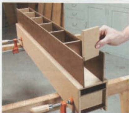
7 Place the sides in the grooves. Apply glue to all four sides of each web piece and stand them in position.
