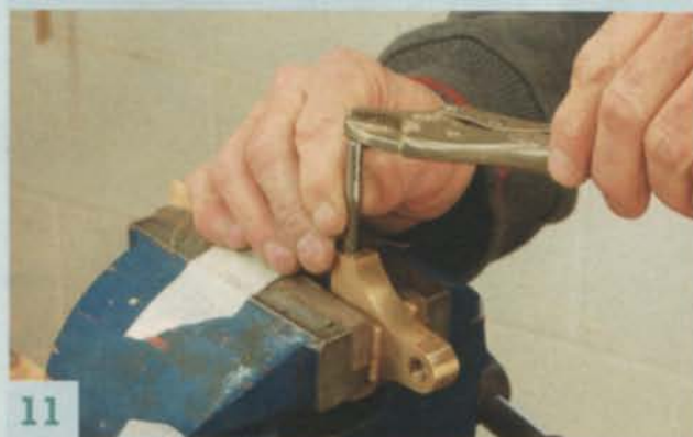
11 Tapping the lever cap was no picnic. In fact, I had to send for a replacement cap, because I mangled the original one.
