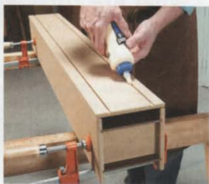
6 Place the second bottom piece on the clamped-up beam. Run a thick bead of glue down both grooves.
