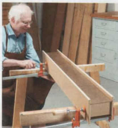
5 Assemble one beam, without glue, and turn it on its side. This creates a level surface for gluing up the other beam.
