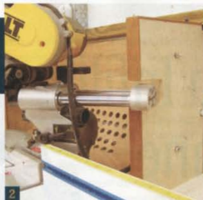
2 A notch in the right end of the box allows the saw's full range of motion.
