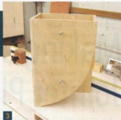
3 An opening in the side of the hose box allows the collection system to draw sawdust through the holes in the curved front.
