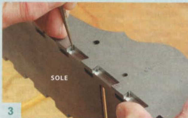
I used the dovetails on the sides to mark the pins on the sole, which were only rough-cut. Filing these joints to fit was pretty easy. However, unlike dovetails in wood, metal dovetails must lock the joint both vertically and horizontally.
