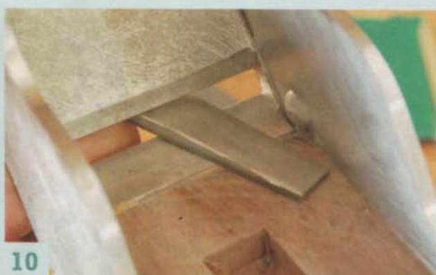
10 Precisely fitting the infill parts was actually enjoyable, because I felt like I knew what I was doing. Here, I'm leveling the bedding surface for the plane iron.
