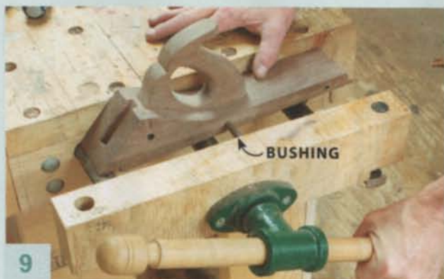
9 Using my vise to press-fit the infill bushings went smoothly. However, drilling rivet holes through the bushings took almost an entire day, and I destroyed a half dozen drill bits in the process.
