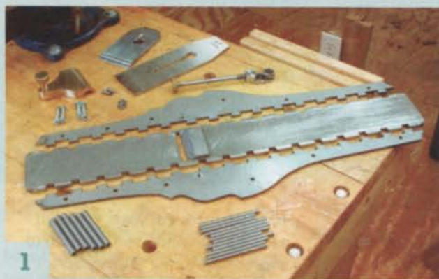
Here's my infill plane kit. Notice that the frog, handle (or tote) and knob (or bun) are missing. These wooden parts comprise the "infill," for which this type of plane is named.
