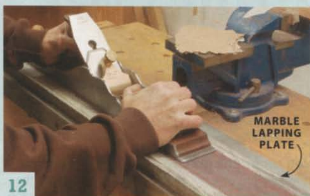
12 Lapping the sole flat took eons, mainly because it was very large and because I stoically kept using sandpaper grits that were too fine.
