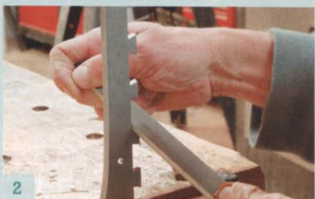
Assembling the dovetailed shell was the first order of business. The laser-cut dovetails on the side pieces cleaned up quickly with a file.
