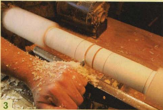
3 Establish the center ring by cutting in with a parting tool.
