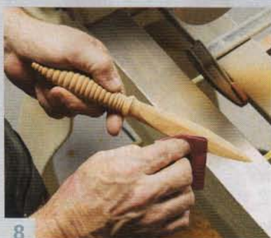
8 Complete the letter opener by sanding with the grain to remove cross-sanding marks from the blade.
