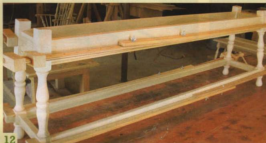
10 To ensure a tight fit , one end of each stretcher has been left unfinished. Clamp each apron between its pair of legs. Then position the stretcher and mark the angled tenon shoulder on the unfinished end.
