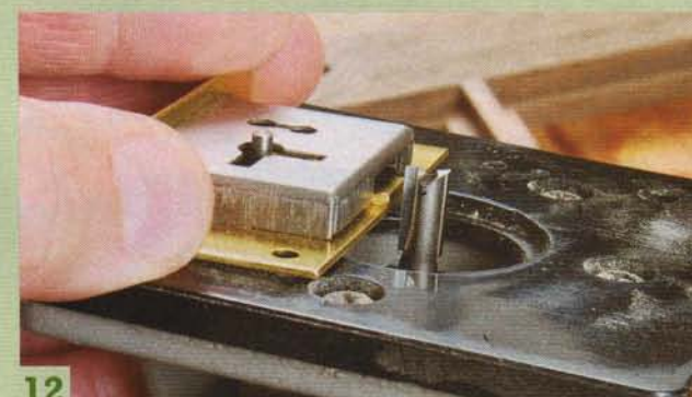
12 Adjust a laminate trimmer slightly deeper than the combined depth of the lock's mechanism and back plate.
