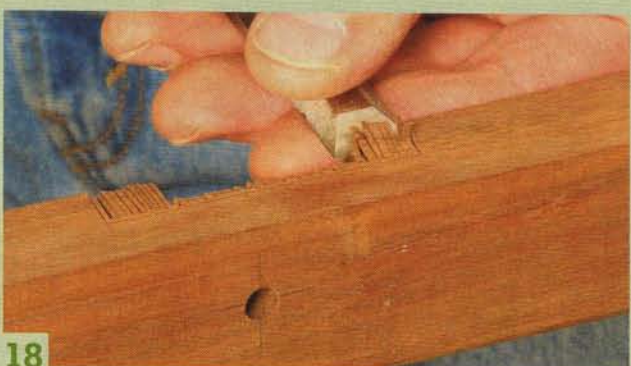
17 To aid in paring this recess, make a series of shallow cuts using a chisel.
