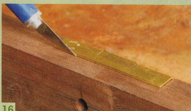
14 Place the lock in the mortise and scribe both sides of the back plate.
