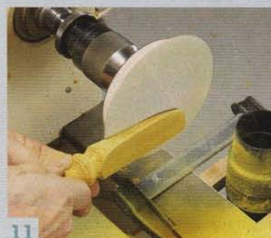
11 The butter knife's blade tapers from the handle to the tip, and from the top to the bottom. Only the bottom edge tapers to a point.
