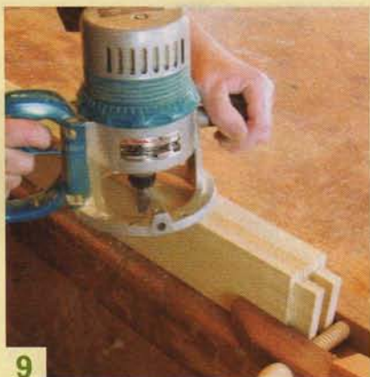
9 Route a bead on the bottom edge of each apron. Gang the aprons together to provide additional support for the router.
