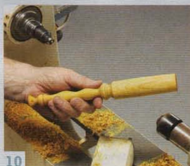
10 Whenever you turn a handle, it's a good idea to stop during the process and check the way it feels in your hand.
