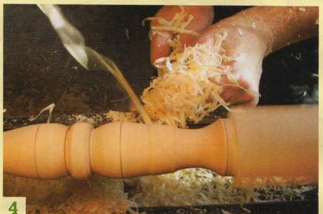
4 Rough out the ring and the vase shapes using a spindle/detail gouge. Shape the vases by eye, using the reference marks you've made. Switch to the skew chisel to finish the job. Use the same tools and techniques to turn the leg's bottom section.
