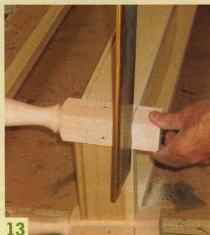
13 Cut the legs flush with the aprons. Then install the pins.
