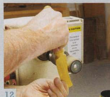
12 Shape the butter knife's blade on a sanding drum, to add interest. A concave curve on the top edge complements the curve on the front at the bottom.
