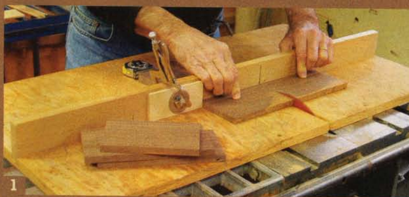
1 Start by preparing the box pieces. A sled and a stop block are great for making repetitive cuts, especially if you're making multiple boxes.
