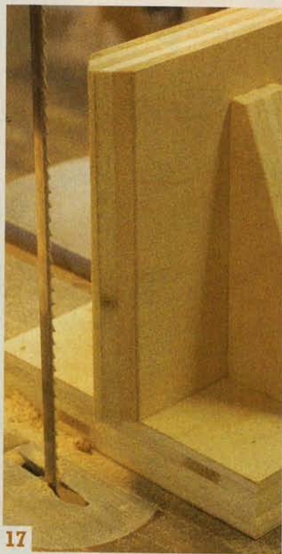
A single-point fence is an alternative to the long fence. It's easier to set up, but you probably won't get an absolutely straight cut.
