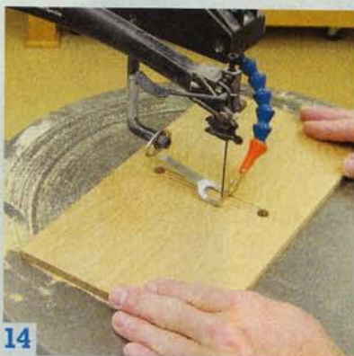
14 Make the door that hides the paper towels. Cut a viewing slot in the door so you can tell when it's time for a refill.
