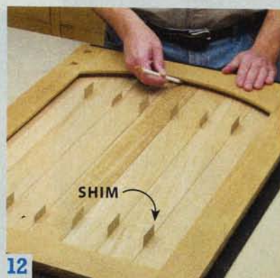
12 Space the slats with cardboard shims, then set the door frame on top. Trace the curve and cut the slats on the bandsaw.
