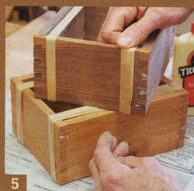
5 Large rubber bands act as clamps and make it easy to remove the squeezed-out glue.
