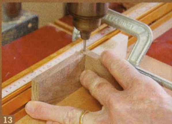
13 Drill the pin hole with the hinge assembled. Advance slowly and carefully, to keep the tiny bit from wandering. Drill slightly over halfway through, then turn the hinge over and drill to the same depth from the opposite end.
