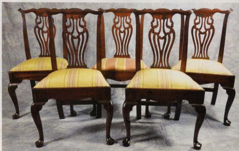
In addition to building these chairs to match a period chair, Janet also installed appropriate upholstery on the slip seats, consisting of silk fabric over loose horsehair and cotton.
