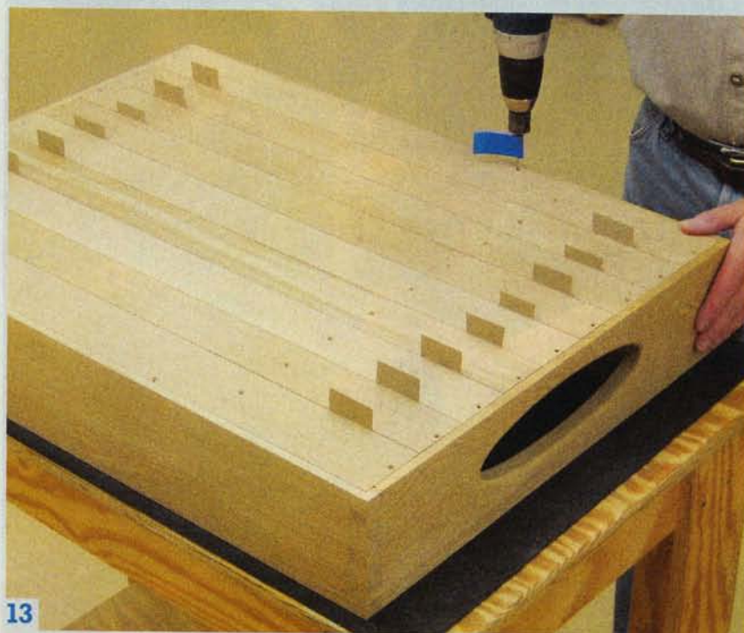
13 Install the slats in the back of the cabinet. Drill pilot holes and fasten the slats with small screws.
