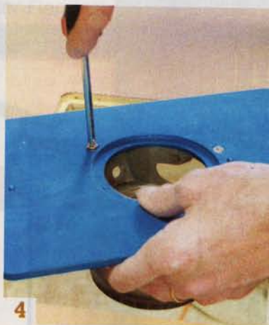
4 Fasten the base from your router to the router plate. Reinstall the router motor and then fit the router plate assembly in the table.
