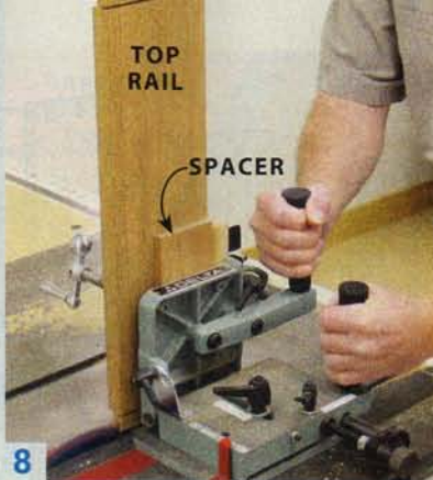
8 Saw tenons on the door's rails using a tenoning jig. You can cut both sides of a tenon, without having to re-adjust the jig, by using a spacer.
