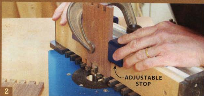
2 Rout tails in the end pieces first, after setting the jig's adjustable stops to correctly hold the workpiece in position. Once the stops are set, routing is a breeze.
