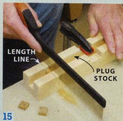
15 Lastly, add the decorative plugs. Saw them in a shop-made miter box. Draw a line on the box to indicate their length.
