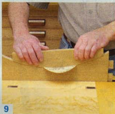
9 Bandsaw an arch in the top rail and sand it smooth. To fair the curve, use the cutoff to hold a piece of self-adhesive sandpaper.
