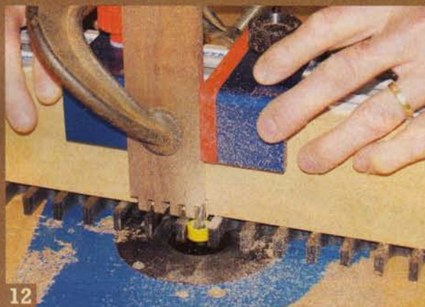
12 Rout the remaining fingers after moving the spacer to the other side of the blank. To create the matching hinge part, simply turn the jig around and repeat the two-step process on the other end of the blank.
