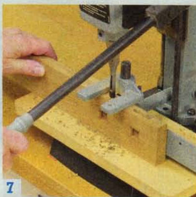
7 Cut mortises in the stiles. Make the mortises slightly deeper than the length of the tenons, to leave room for excess glue.
