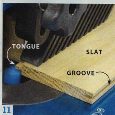
11 Make slats for the back of the door and the back of the cabinet. Rout tongues on the slats using a straight bit.
