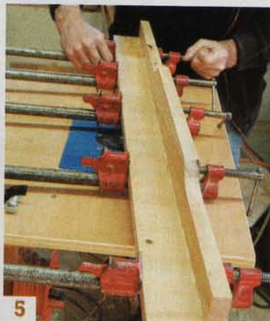
5 Assemble the pivot fence with biscuits and glue. Make sure the joint is flush on the bottom when you clamp the parts together.
