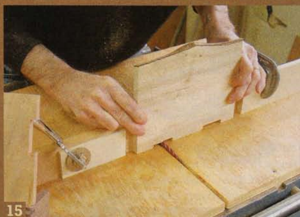
15 Cut notches for the hinges in the back edge of the lid, using a pair of stop blocks and multiple passes. After cutting the first notch, flip the lid around to cut the second notch.
