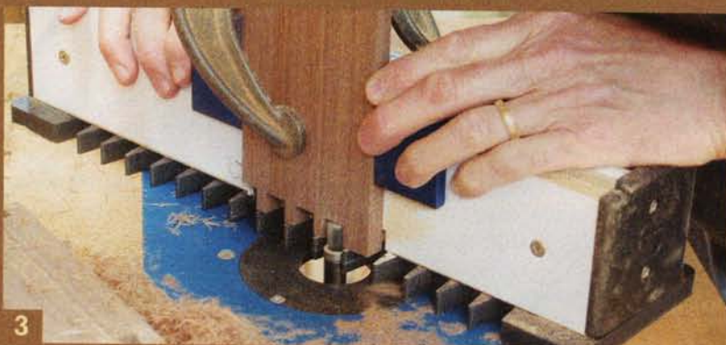
3 To rout pins in the side pieces, simply change to a straight bit and turn the jig around. The stops automatically position each workpiece correctly.
