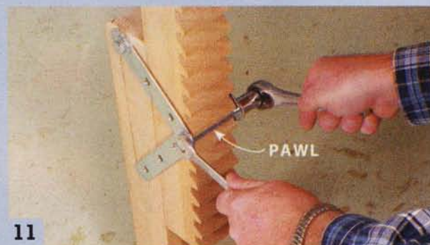
11 Mount the ratchet arms to the lower legs. Add a bolt between the arms as a pawl to engage the ratchets.
