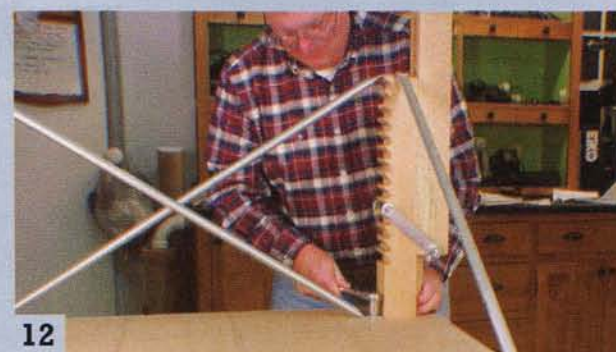
12 To make the legs extra-sturdy, add braces made from electrical conduit.
