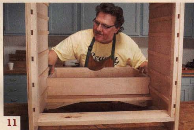
11 Check the fit. If the drawer is too tight, remove both runners and shave a bit of thickness from each one. Reinstall the runners and try again. Keep removing and shaving until the drawers slide freely.
