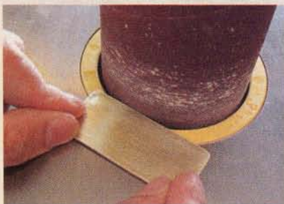
7. Cut out the blank and smooth the edges.
