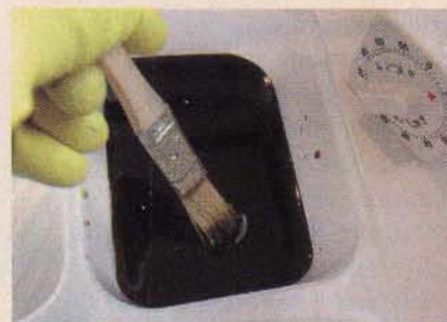
12. Cover the blank with acid , brush it occasionally, and let it soak. After a while, check the edge of the mask with a toothpick. Eventually, you'll be able to feel a ridge.
