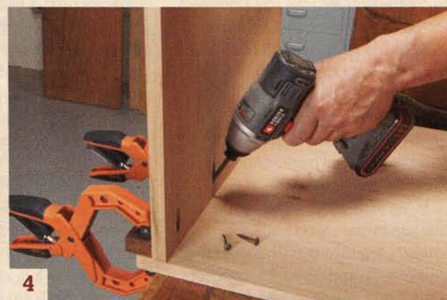
4 Fasten the sides to the top with glue, biscuits and screws. Clamp a fence to the outside edge of the top, to hold the side in position as you drive in the pocket screws.
