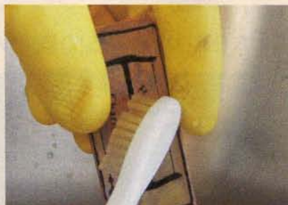
14. Tone the brass by brushing on a metal darkening solution.
