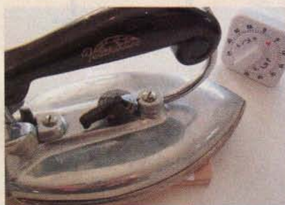
10. Use heat to transfer the image from the film to the blank. Once it's transferred, the toner ink mask will resist the acid used to etch the brass.
