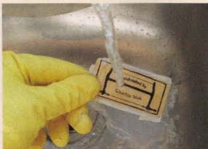
13. Remove the etched blank from the acid and thoroughly rinse it.
