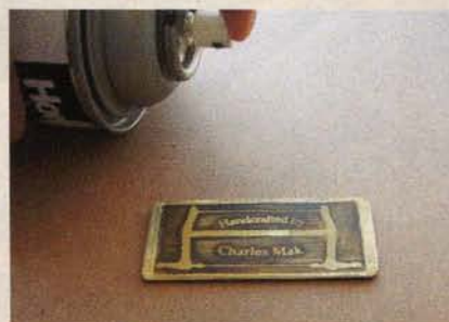
16. Seal the nameplate's etched and patinated surface with lacquer.
