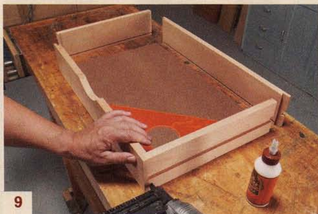
9 Assemble the drawers with glue and brad nails. Check each joint to make sure the drawer is square.
