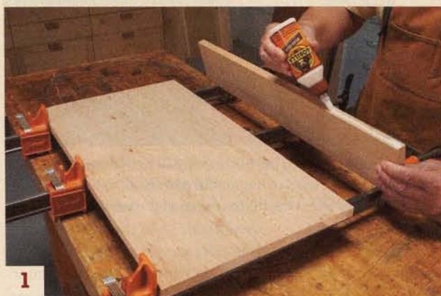
1 Glue up the panels for the sides and top. Work on a flat surface and glue the joints one at a time.
