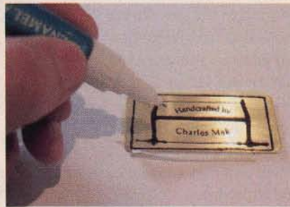
11. Touch up the transferred mask , after letting the blank cool and peeling off the transfer film. You can add color where it's missing, or remove color where it isn't wanted.
