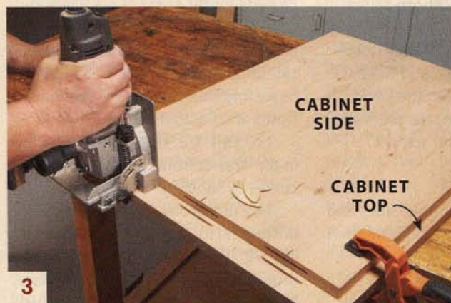
3 Cut biscuit slots in the top and sides. Then drill holes for pocket screws on the inside face of each side.
