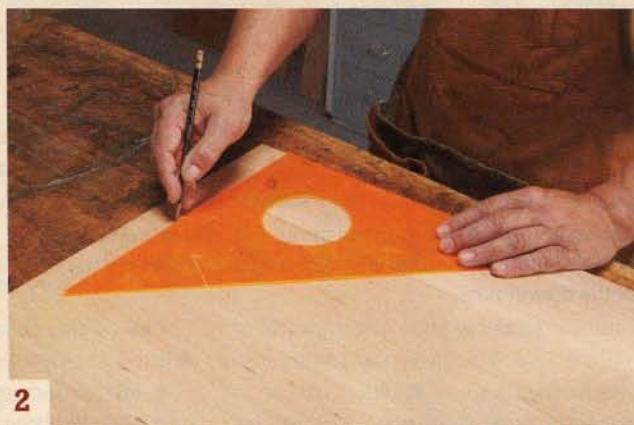
2 Mark the location of the sides' inside edges on the top's bottom face. Use a large square for accuracy.
