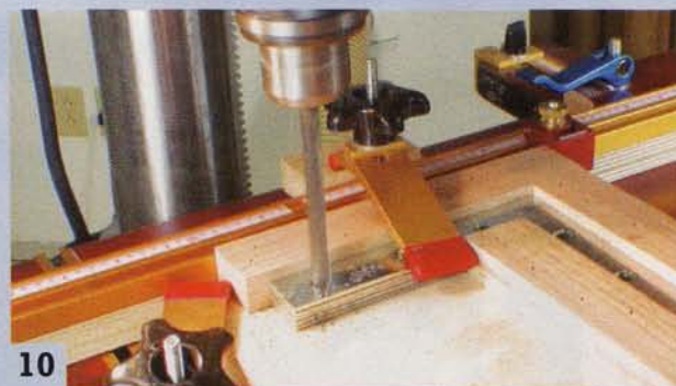
10 Make four ratchet arms from ordinary flat corner braces. Drill identically-spaced holes in the braces by stacking the pieces in a jig.
