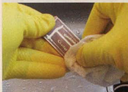
15. Remove the mask by rubbing the blank with a soft cloth dampened with acetone.
