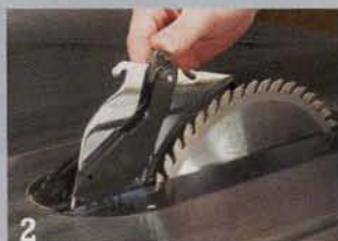
Installing the blade guard assembly takes only seconds. First, pull the release lever to raise the riving knife (1). Then snap in the anti-kickback pawls (2). Hook the guard assembly on the riving knife (3) and lock it in place (4).
