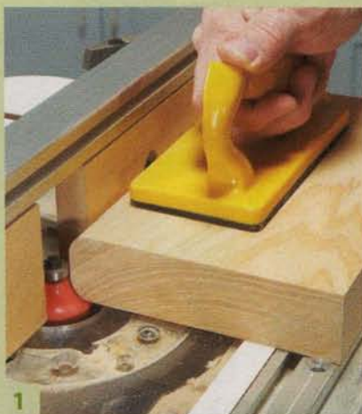
1 Round over one side of a squared-up blank, to duplicate the look of a book's spine.
