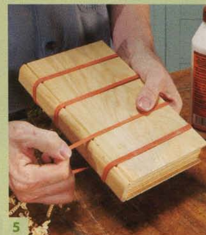
5 Glue the spine back to the body. Use rubber bands as clamps to avoid marring the book.
