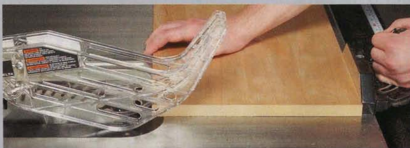
The new Unisaw's table is significantly longer in front of the blade, a boon to both ripping and crosscutting operations.
