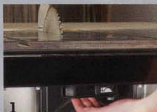
Installing the blade guard assembly takes only seconds. First, pull the release lever to raise the riving knife (1). Then snap in the anti-kickback pawls (2). Hook the guard assembly on the riving knife (3) and lock it in place (4).
