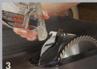
Installing the blade guard assembly takes only seconds. First, pull the release lever to raise the riving knife (1). Then snap in the anti-kickback pawls (2). Hook the guard assembly on the riving knife (3) and lock it in place (4).
