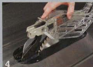
Installing the blade guard assembly takes only seconds. First, pull the release lever to raise the riving knife (1). Then snap in the anti-kickback pawls (2). Hook the guard assembly on the riving knife (3) and lock it in place (4).
