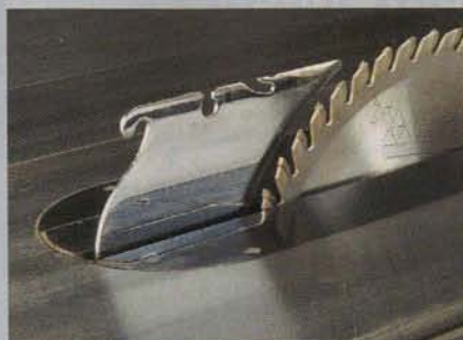
The riving knife reduces the likelihood of a kickback. It sits below the blade, so you don't have to remove it for non-through cuts, and it travels with the blade during adjustments, so it's always perfectly positioned.
