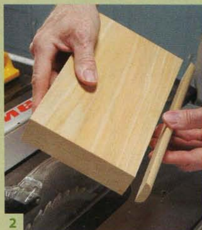
2 Rip the blank to separate the spine from the body of the book.
