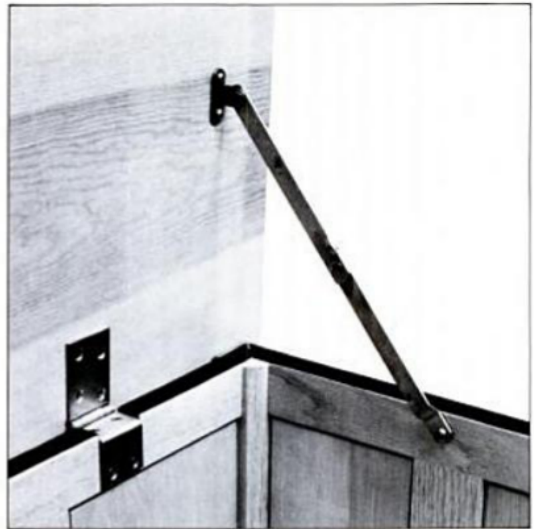
The hinge is flush-mounted on the lid and inside surface of the rail and set into the top edge of the rail.
