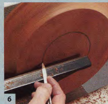
6 Mark a circle slightly larger than the faceplate on the spinning blank. Then remove the blank from the lathe, and the faceplate from the blank.
