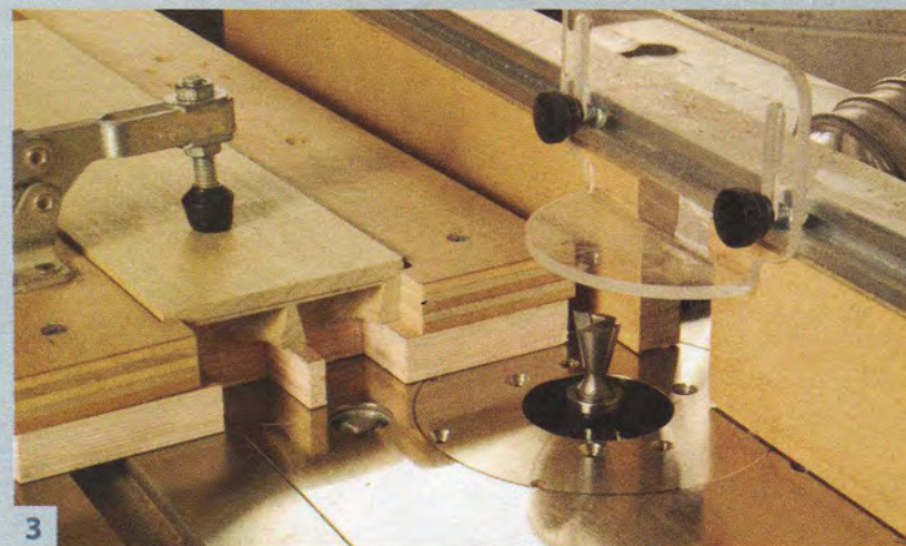
3 Precision joints can also be made with shop-made templates. I designed this template for routing half-blind dovetails in a drawer front.
