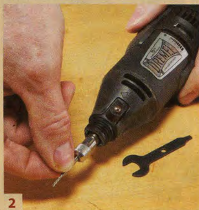
2 Install a 1/16" bit in a Dremel or small router. If you're using a Dremel, mount it in a Dremel plunge-router base.
