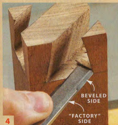
4 To pare cleanly into the acutely angled corners, bevel the sides of your chisel.
