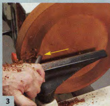
3 Flatten the back side of the blank. Work from the center to the outside. Start with the bowl gouge; then switch to a square-ended scraper to level the surface.
