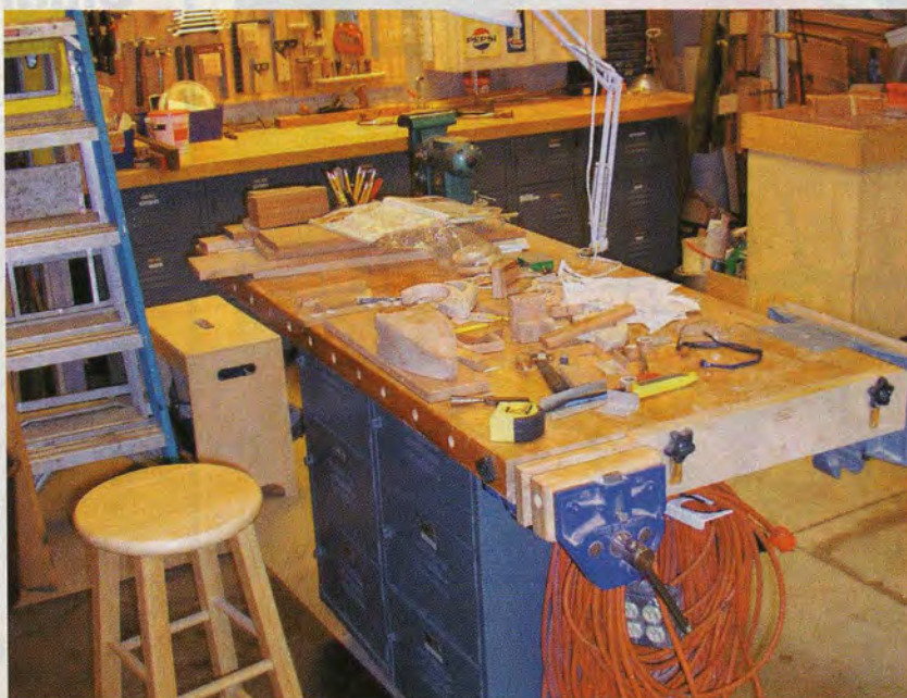
My workbench tops were salvaged from an old junior high school. They're mounted on old steel storage lockers and fitted with locking casters.
