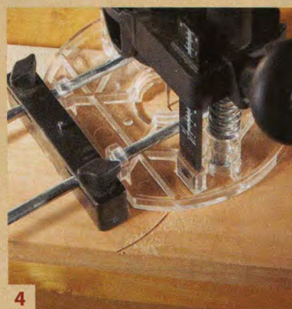
4 Adjust the bit to make a cut 1/32" deep. Make a shallow hole with an awl. Hammer the nail into the hole, and make a test pass.
