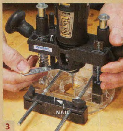
3 Add an adjustable fence to the base, which includes a pivoting point (a 3d nail). Adjust the distance between the bit and nail to the radius of the arc that your design requires.
