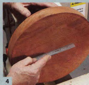
4 Use a straightedge to check the leveled surface. The center area must be absolutely flat, so you can successfully remount the faceplate when it's time to turn the plate's open side.
