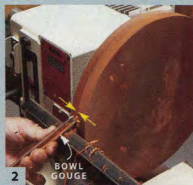
2 Use a bowl gouge to true up the edge of the blank and make it round. Avoid splintering the blank's faces by working the edge from both sides. Start at the outside and move to the center.
