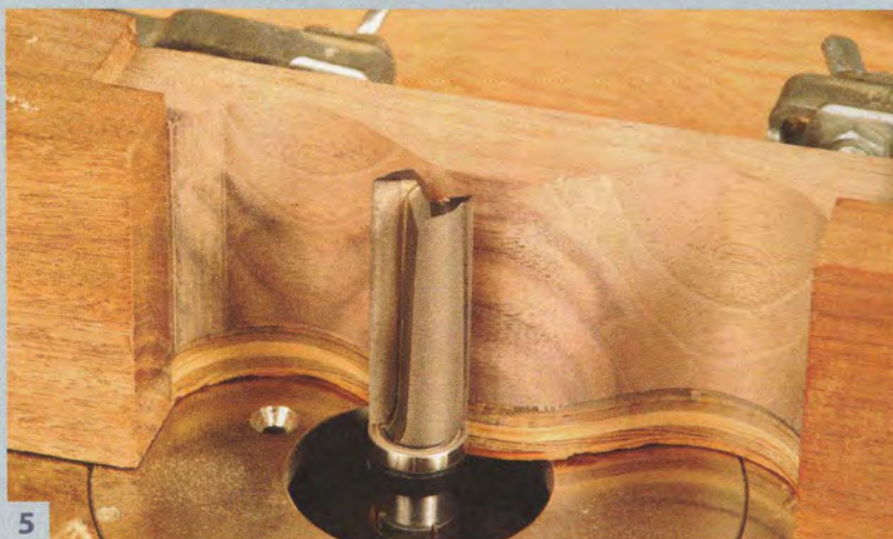
Curved parts, both large and small, can be duplicated by template routing. Here, I'm using a tall flush-trim bit to shape a small serpentine drawer front.
