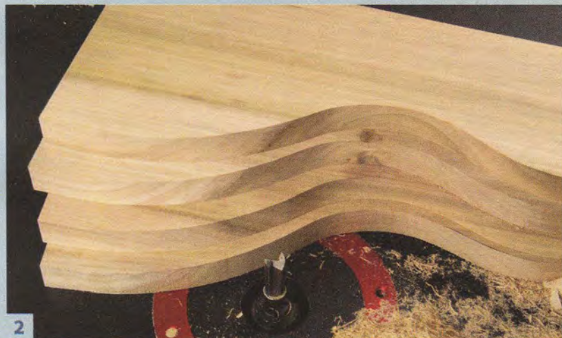
2 Identical parts with smooth, uniform surfaces are easy to make using a template.
