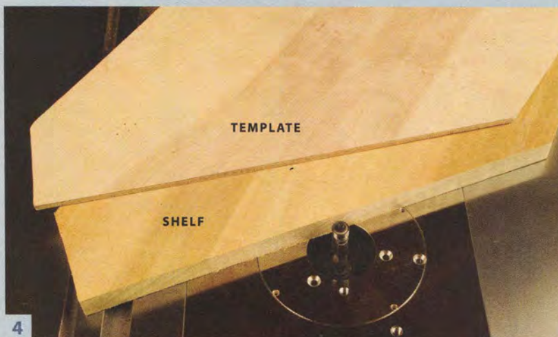
A straight cut that's not parallel to another side is hard to set up on a tablesaw, so it's an ideal candidate for template routing. This is a diamond-shaped shelf for a corner cupboard.
