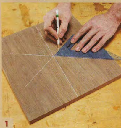
1 Begin by drawing centering lines on your workpiece. First, draw a slightly offset vertical line in the center. Next, draw four lines radiating at 60°.
