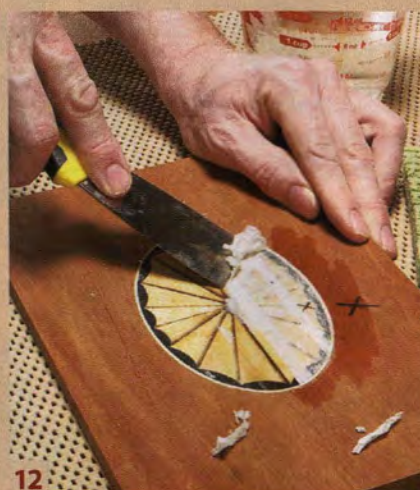
12 Remove the tape by moistening it with a sponge. Wait a minute or two, then scrape off the tape using a dull putty knife.
