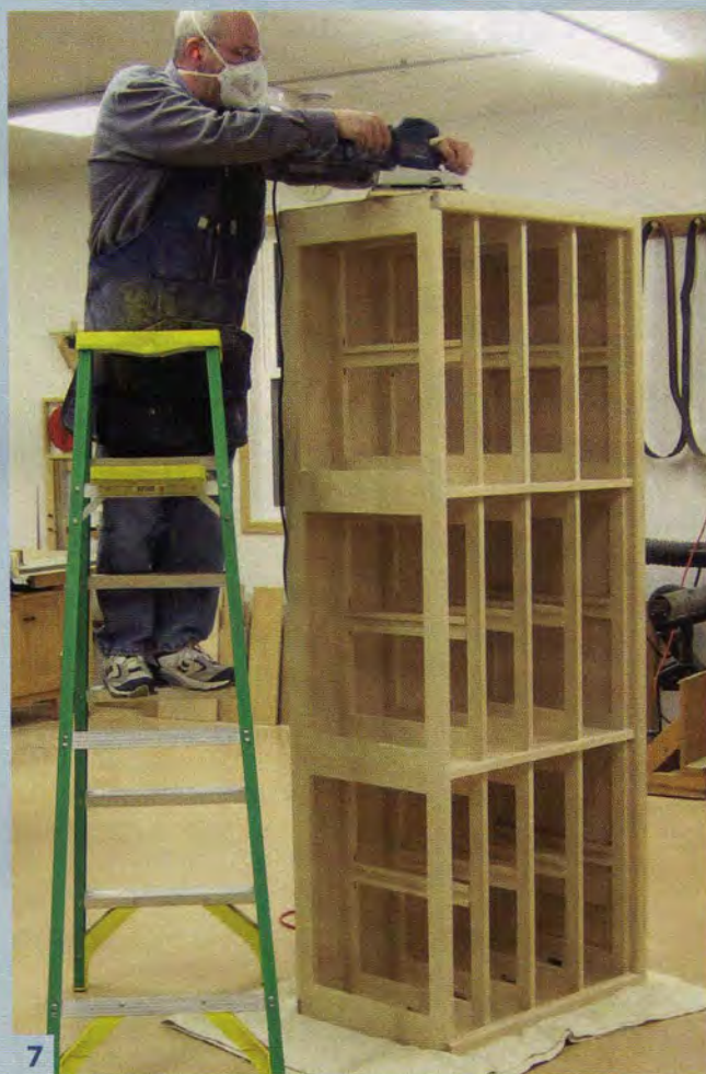
7 Use an orbital sander to sand the cabinet's ends. An orbital sander is not as aggressive as a random orbit sander and gives a better final finish.
