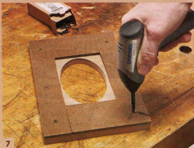
7 Fasten a shim piece to the template's bottom side. The thickness of this piece is determined by the length of your router bit's cutting flutes.
