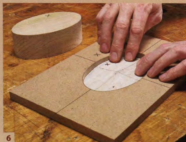
6 Check your progress by placing the oval in the template's window. Aim for a snug fit, with no gaps.
