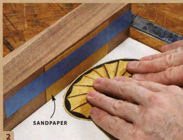
2 Remove remaining bits of border material by sanding the oval on a right-angled block. This ensures that the oval's edges are square.
