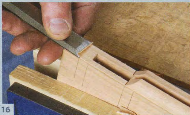
16 Pare the remaining waste. Go down to the sticking's inside edge on the front and the scribe mark on the back.
