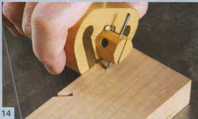
14 Set a marking gauge to the width of the sticking and scribe a line on the stile's back, behind the mortise.
