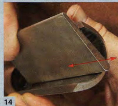
14 Use the slipstone's rounded edge to hone the inside. Hold the slipstone flat in the flute and move in an out, following the flute's curve, without tipping forward over the edge.
