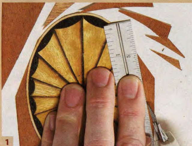
1 Some inlays have a rectangular border which must be removed. Cut off the border using a sharp knife guided by a metal straightedge.
