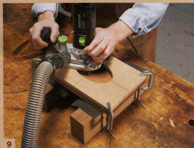
9 Clamp the template to the workpiece and rout a recess for the inlay. Using this bit, the recess will be exactly the same size as the template's window.
