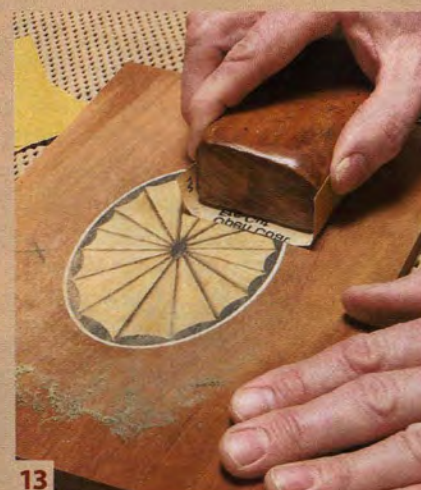
13 Sand the inlay flush with the surrounding wood. Use 220 grit paper wrapped around a cork-backed block.
