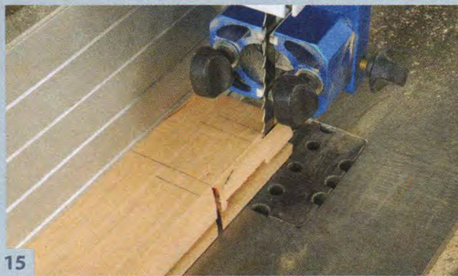
15 Remove the waste by sawing close to the sticking's edge or the scribed line, depending on which end of the stile you're cutting. Guide the cut with a fence.
