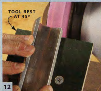
12 To sharpen the tool, grind a 45° bevel behind the edge. Hold the tool parallel with the wheel's edge and flat on the tool rest. Then roll it slowly from corner to corner. Stop grinding when the sparks appear evenly along the edge.
