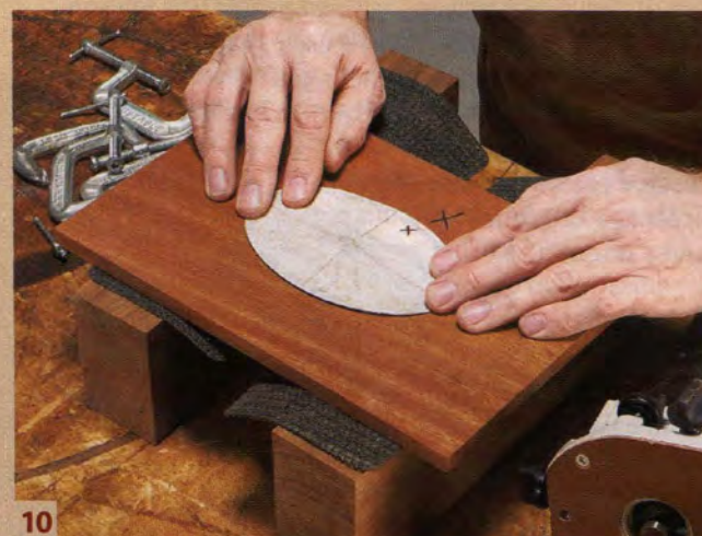
10 Test the fit of the inlay in the recess. If the inlay is too large in spots, sand those areas using the right-angle sanding block.
