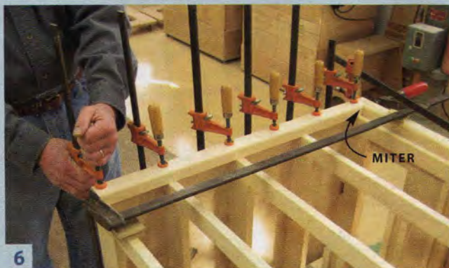
6 Glue edging onto the front of the cabinet. The edging is mitered at the corners, down at the base. Draw the miters tight with long clamps.
