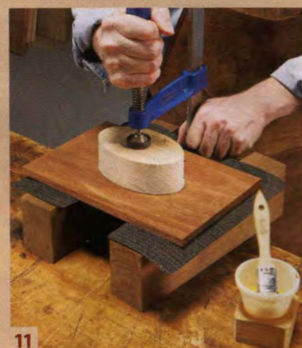
11 Glue the inlay. Apply even pressure by using a thick block that's just a bit smaller than the inlay.
