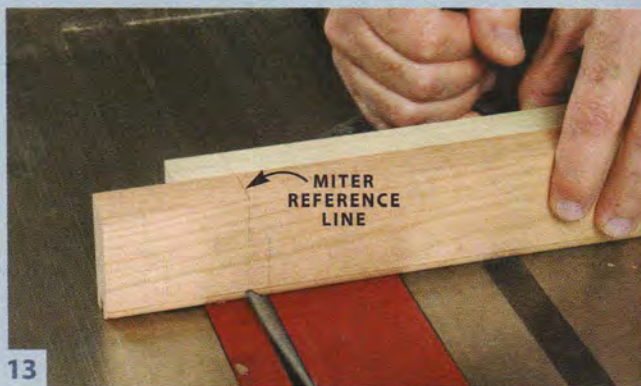
13 Miter the stile by aligning its miter reference line with the reference line on the backing board.
