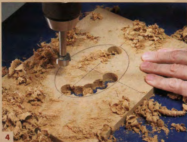
4 Remove most of the waste inside the oval using a Forstner bit in the drill press.
