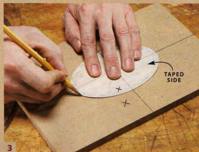
3 Make a router template from MDF. Turn over the inlay, taped side up (this is the show side), and trace around it.
