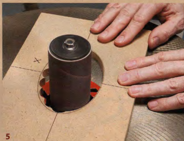
5 Sand up to the pencil line using an oscillating spindle sander or a sanding drum in your drill press.
