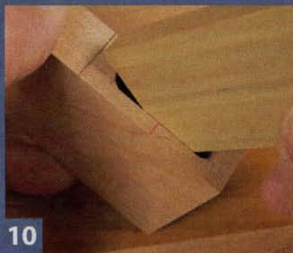
10 Size a loose tenon blank. Plane a length of stock to fit the mortises. It should slip in without wiggling or binding. Rip the blank to width, slightly less than the mortises' length.
