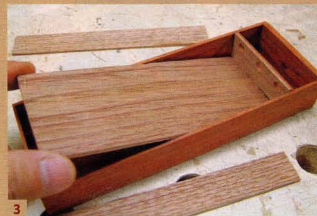
Remove the inner box from the outer box and line it with Spanish cedar. Be sure to use water-resistant glue.
