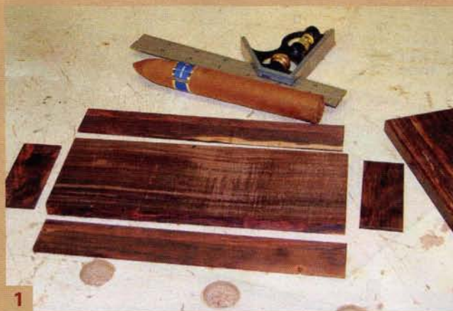
Build the outer box from a single piece of Brazilian rosewood that's been resawn into thin boards. Size the pieces to fit the objects you'll be carrying.
