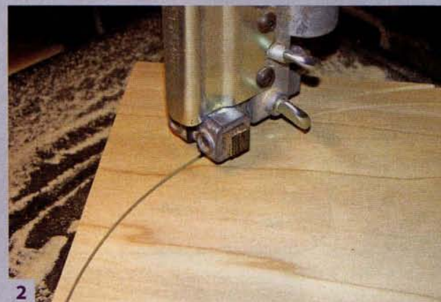
2 Saw the round board on the bandsaw, using the circle-cutting jig. I usually make two passes around to make sure no high spots remain. Sand the edge to remove the saw marks.
