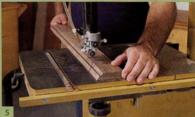
5 Build a jig for routing the second bevel. Rout a lock miter on this piece by standing it on edge, as in the last step. Remove the center portion of the lock miter profile using a bandsaw.
