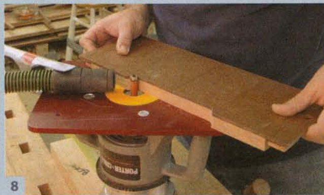
Make hardboard templates for the rails, then shape the rails using a flush-trim bit. You can see that my router table is very simple!
