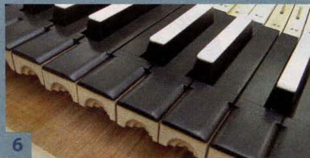
6 Walnut, ebony and bone are laminated to the tops of keys for durability and appearance.
