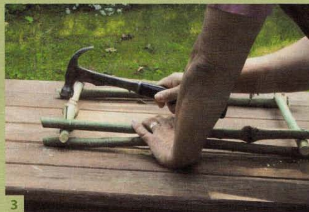
Nail each frame together after pre-drilling each hole, to avoid splitting the wood. Orient the pieces firmly against the bench, so the force of the hammer is directly transferred through the nail to the bench.
