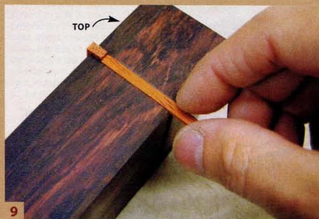
9 Install the inlays. Start with the top piece, then add the side pieces. Fit the bottom inlay last, to minimize exposed end grain.
