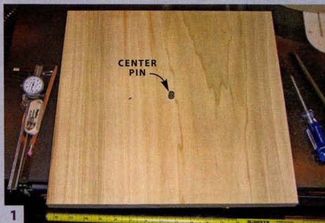
1 Start by cutting a square blank slightly larger than the game board's diameter. Install a nail or pin at the center for use with a circle-cutting jig. The nail hole will disappear when you rout the center marble pocket.
