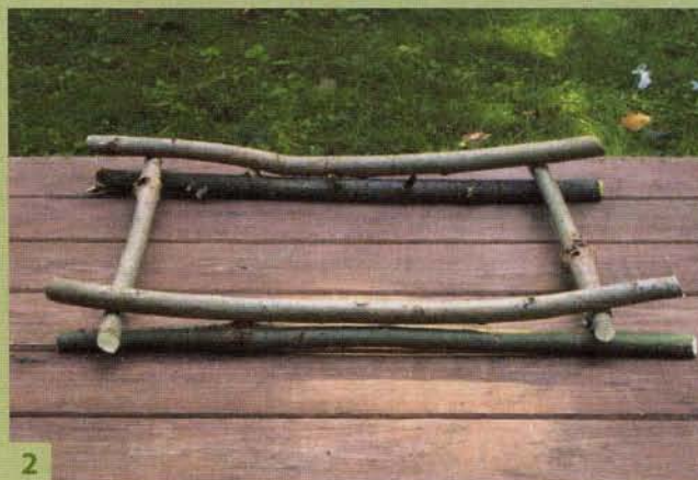
Start by making a pair of frames. One frame supports the seat; the other frame supports the legs. Using a slightly curved branch for the front of the seat frame makes the seat more comfortable.
