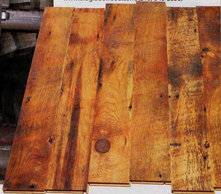
9 Cleared of nails, the wood is resawn and milled into boards for flooring and paneling.
