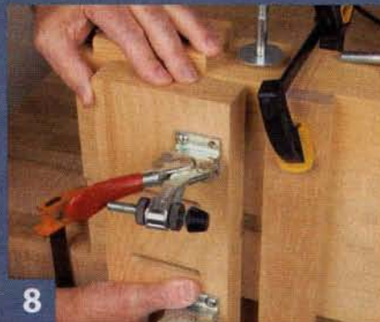
8 To mount the vertical holder, clamp a workpiece with its mortise centerline aligned with the jig's registration line. Slide the holder against the workpiece and tighten the bolts.
