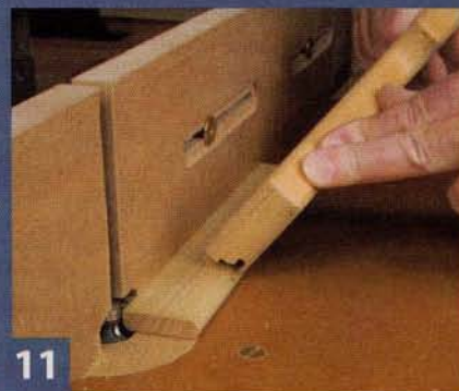
11 Round the tenon blank's edges to match the mortises. Then cut individual loose tenons from the blank.
