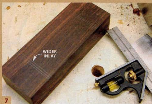
7 Lay out the inlays on the box after the lid is glued on. The inlay on the humidifier end of the box (the end with the washer) is 1/16" wider. The extra width will be removed when the box is cut open.
