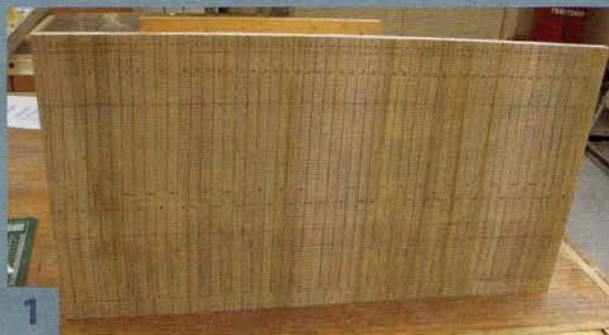
1 The keyboard building process begins by gluing up a poplar panel large enough to accommodate an entire keyboard.
