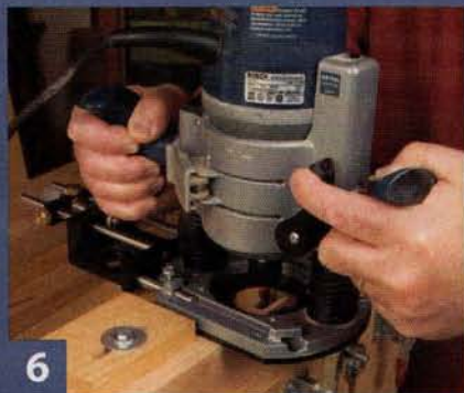
6 Rout the mortise with a series of shallow cuts. Plunge the bit about 1/8" and feed quickly to the far stop. Retract the bit, return to the starting position and go again.
