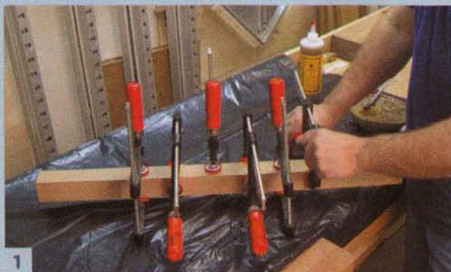
1 Begin by gluing up the legs. Each leg is composed of four pieces of quartersawn oak, joined by lock miters. (For more on this technique, see Four-Sided Quartersawn Table Legs, page 47).
