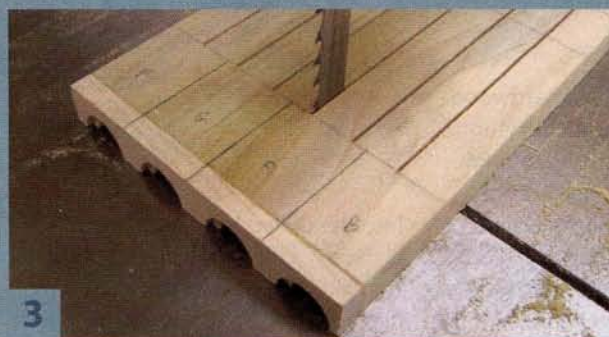
3 A bandsaw and scrollsaw are used to cut the blank into individual keys. Straight "sharp" keys lie between pairs of square-shouldered "natural" keys. The scroll saw cuts the square shoulders.
