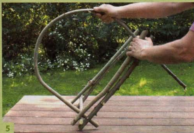
5 Bend the arm inside the opposite rail and nail it in place. Then trim the ends. This chair has a total of four bent arms. Pre-bending the branches before installation makes their curves more uniform.
