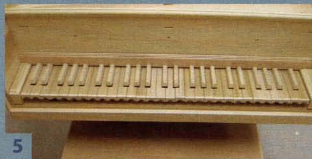
5 Once the keyboard has been completed, the entire assembly is fitted into the case
