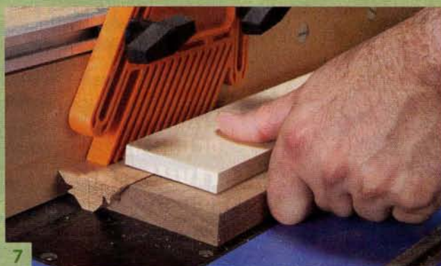
7 Rout the second bevel with the workpiece held horizontally. The jig provides a wide bearing surface in order to cut a perfect joint on this narrow piece.
