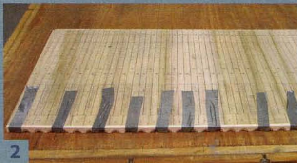
2 The decorative key tips (called arcades) are applied as a single strip to the keyboard blank before the blank is sawn, first into sections, and then into individual keys.
