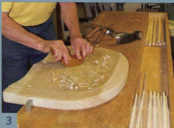
Wallace completes the scooping using a travisher—a wooden convex spokeshave—followed by a random orbital sander.
