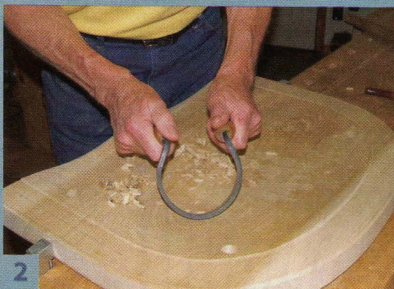
The smoothing process continues with an inshave. Many of the tools used during the process evolved out of the wheelwright's trade.
