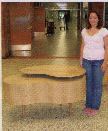
Brienna Larrick shows off a project she completed through a WoodLINKS program. She designed the piece with AutoCAD and cut out the shapes with a CNC router. After assembling the curved honeycomb structure, she used a vacuum press to glue on the face veneers.
