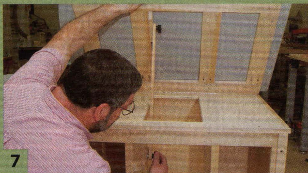
7 Build an arm to prop the top. This makes it much easier to change bits because there will be plenty of elbowroom around the router. Plus, you don't have to bend over.
