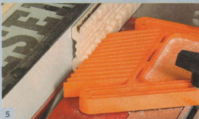
Begin making the sockets by removing some of the waste on the tablesaw.
