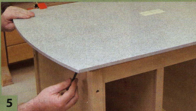
5 Clamp the top to the base and trace all the way around the top's underside. Turn the top over.
