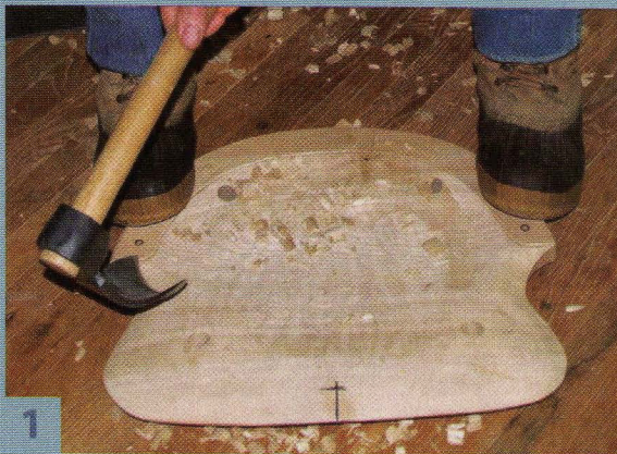
After bandsawing the seat blank to shape, Wallace uses a gutter adze to roughly contour the scooped seat. Except for a few guide marks, Wallace performs the entire process by eye.
