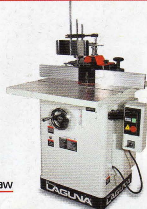
Platinum Series Shaper Deluxe Fence w/ Micro-adjust 3-hp Leeson Motor 3/4" & 1" Spindle Included 1/4" & 1/2" Router Collet - Included
