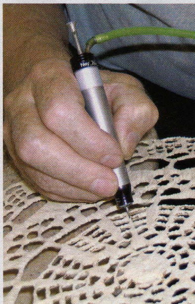
Darwin uses a slow-speed (100,000 rpm) rotary tool to carve large pieces, such as the telephone in "Missing You" (see page 28).
