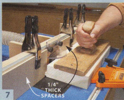
Route the profile in two passes. Clamp spacers to the fence to limit the cut on the first pass. Routing this profile in a single pass removes too much material.
