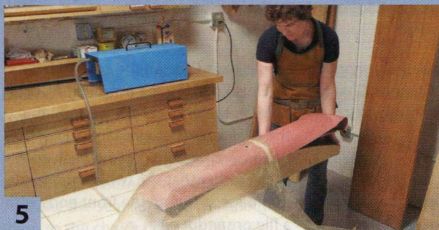
5 Place the laminations on the bending form, cover them with paper to absorb any glue squeeze-out, and slide the assembly inside a vacuum-veneer bag.
