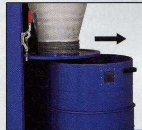
Step 2 Remove Drum
