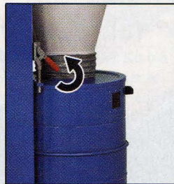
Step 1 Lift Drum Lever
