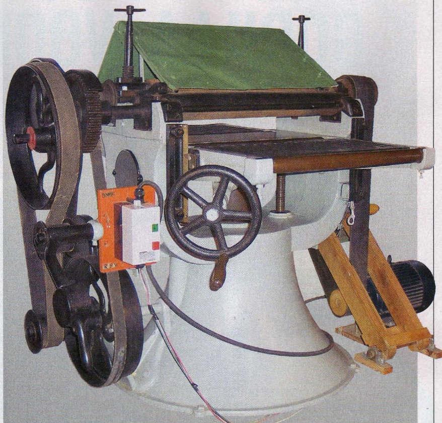
After restoration, my 1876 planer still runs on flat belts, but I power it with an electric motor. The bed is supported by a single column, housed in the bell-shaped base.
