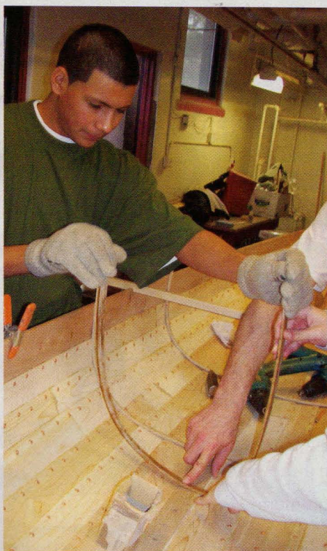
Mario fitting steam-bent rib into canoe.
