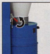
Step 1 Lift Drum Lever
