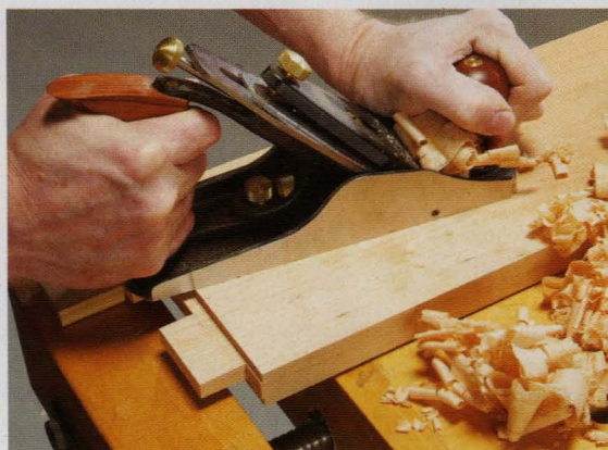
Smoothing planes take the place of power sanders. They're used for making a surface ultra-smooth and ready for finishing.
