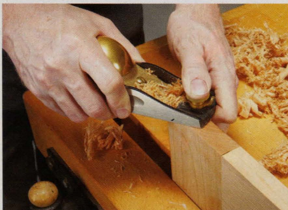
Block planes are designed for cutting end grain, such as the stile of this door frame. Their compact size also makes them perfect for planing with one hand.
