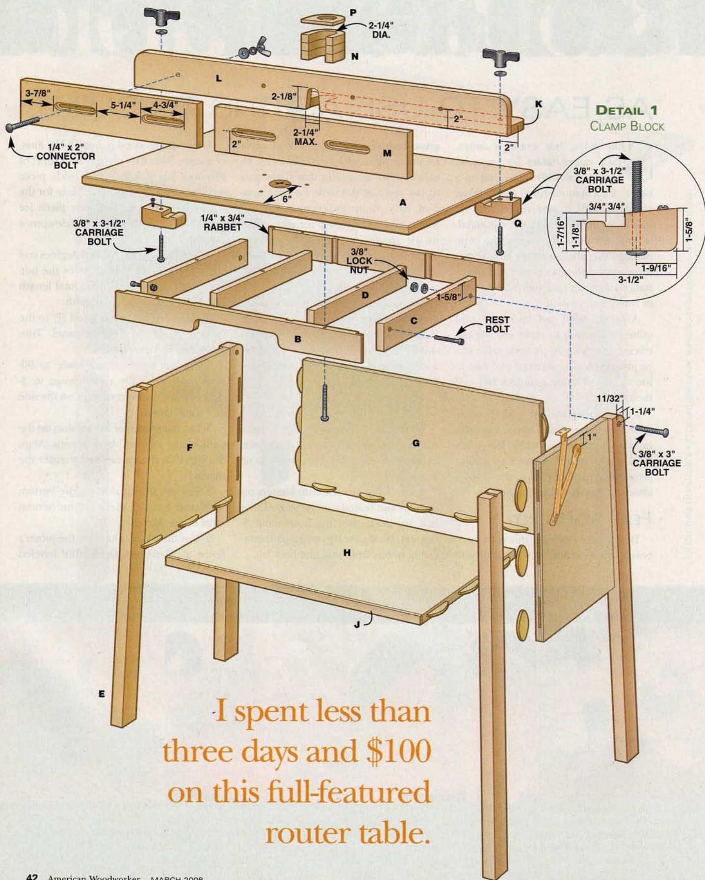
FIGURE A EXPLODED VIEW
