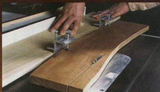
Straighten crooked boards in two passes
