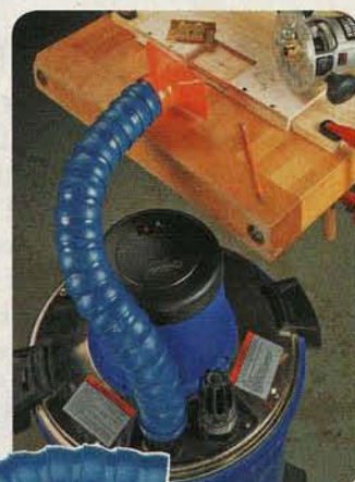
Loc-Line® hose with vacuum adapter connected to shop vacuum.
