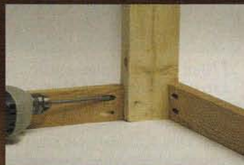
Assemble flush & corner joints
