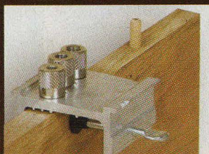
Pre-aligned drill stops for 5/8", 3/4", & 1" stock
