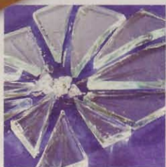
Plate glass shatters into razor sharp shards when it breaks.
