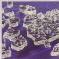
When tempered glass does break it crumbles into cubes.
