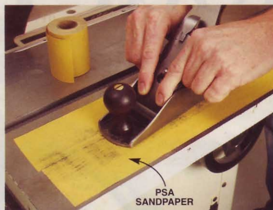
Flatten your plane's sole using sandpaper. A flat sole enables a plane to make long, thin shavings.
