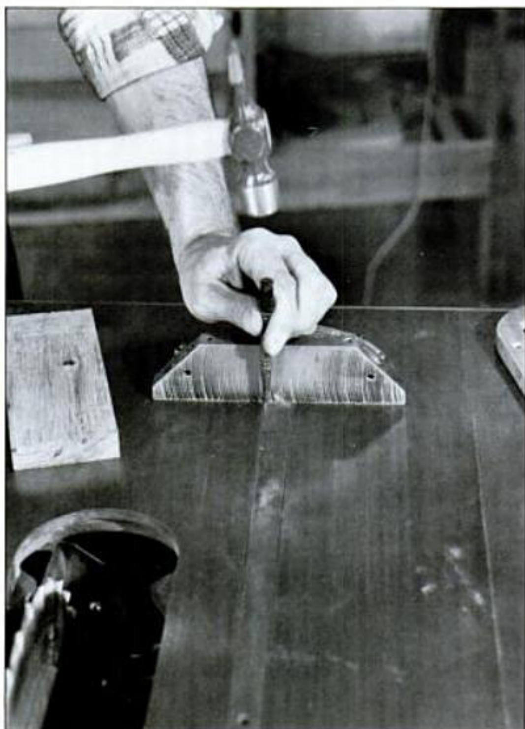
A tap with a center punch on the edge of the miter-gauge bar will tighten up excess side-to-side play.
