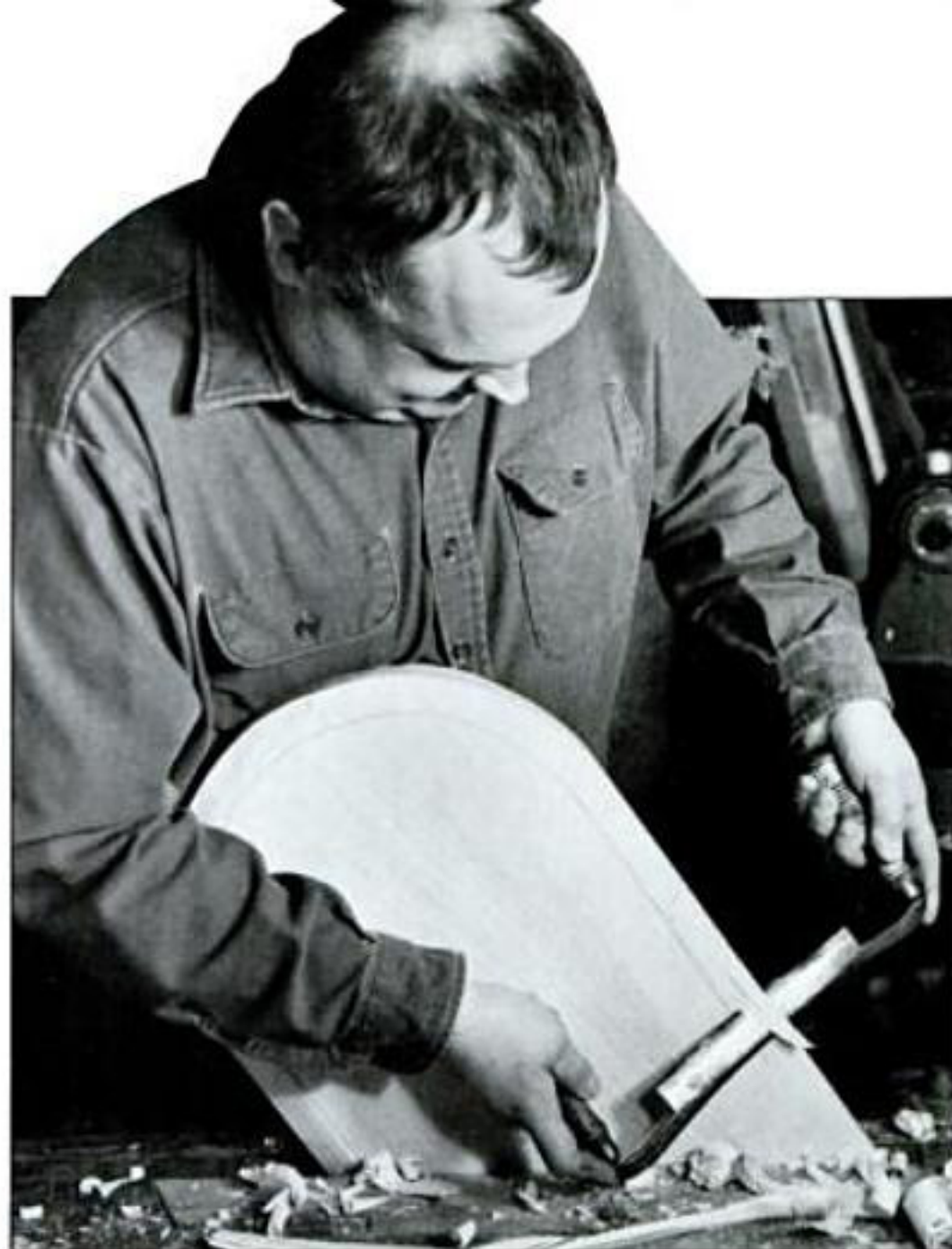
Mark off a bevel around the underside of the cradle bottom, and remove the bulk of the wood with a drawknife.
