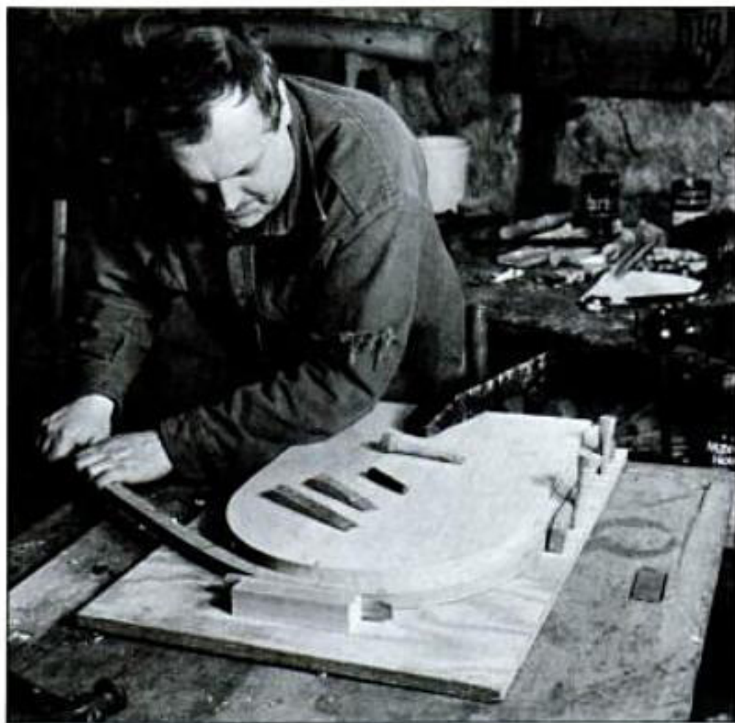
Hot stuff. Bend the steam-softened rail around the bending form, and clamp it in place with wedges between the dowels and the rail.
