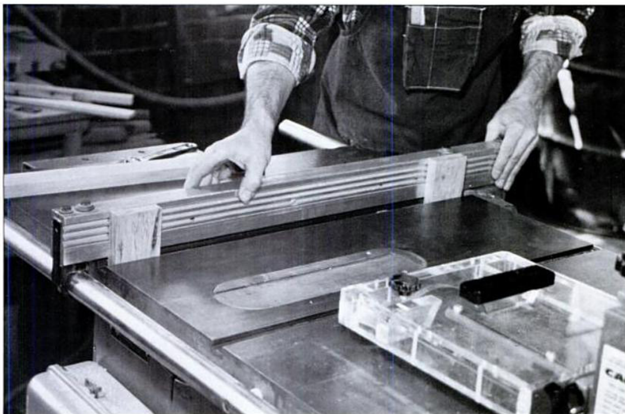
An easy way to align the fence with the miter-gauge slot is to insert two pieces of wood in the slot, and lock the fence against the wood.
