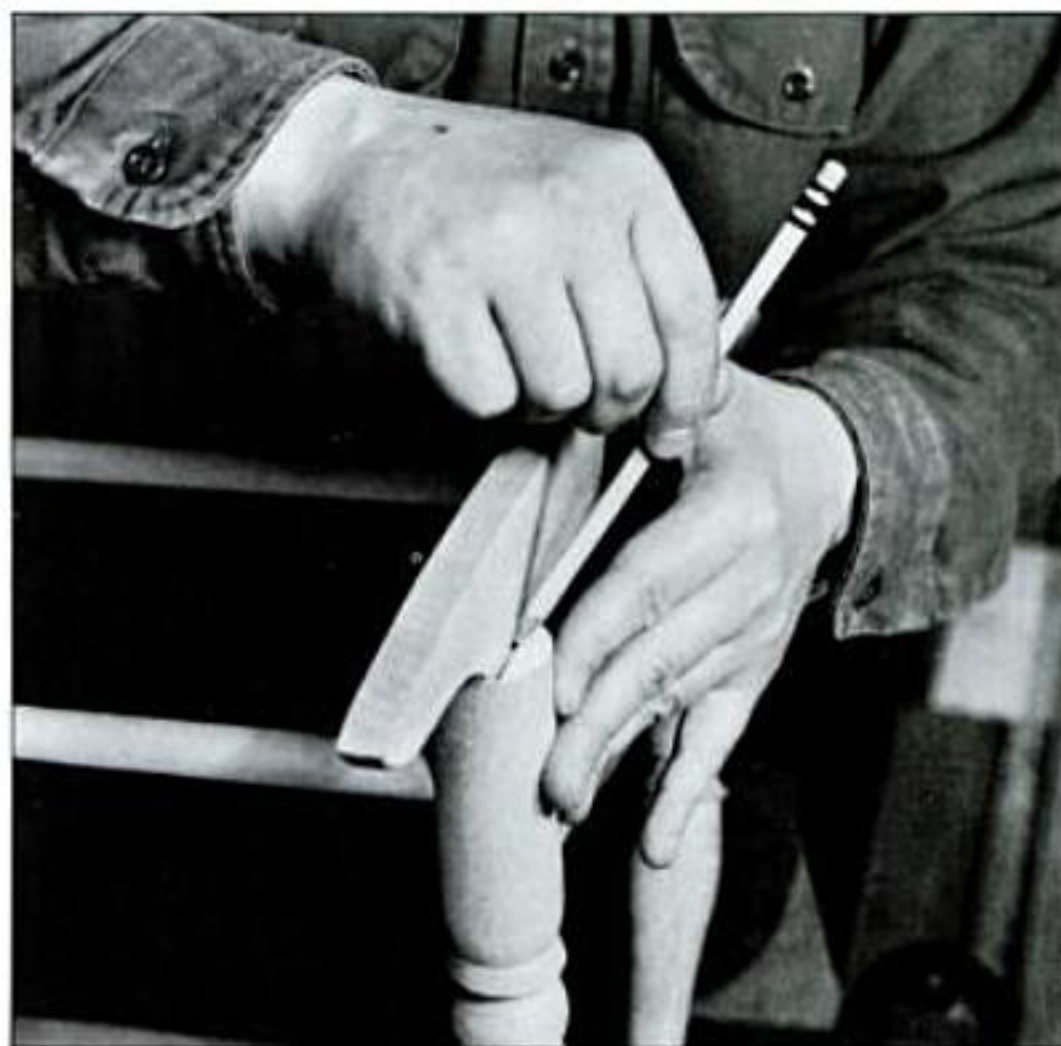
With the legs and stretchers assembled, mark off the slot for the rocker, and extend the marks down the legs with a square.
