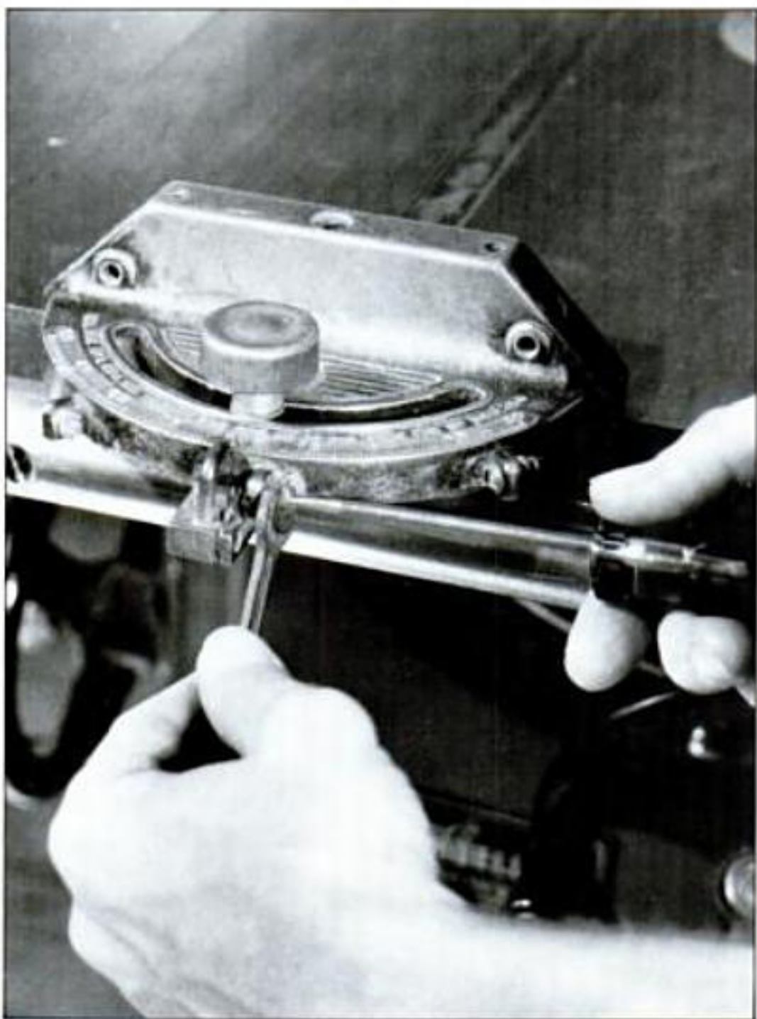
Set the miter-gauge stops with a wrench and a screwdriver.
