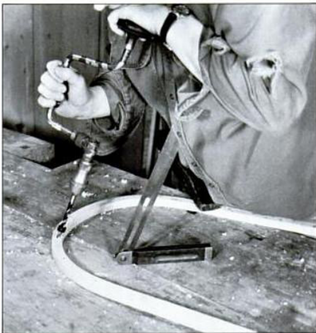
Drilling angled holes like those for the spindles and legs is easy if you line up the bit with the blade of a sliding bevel placed next to the hole.
