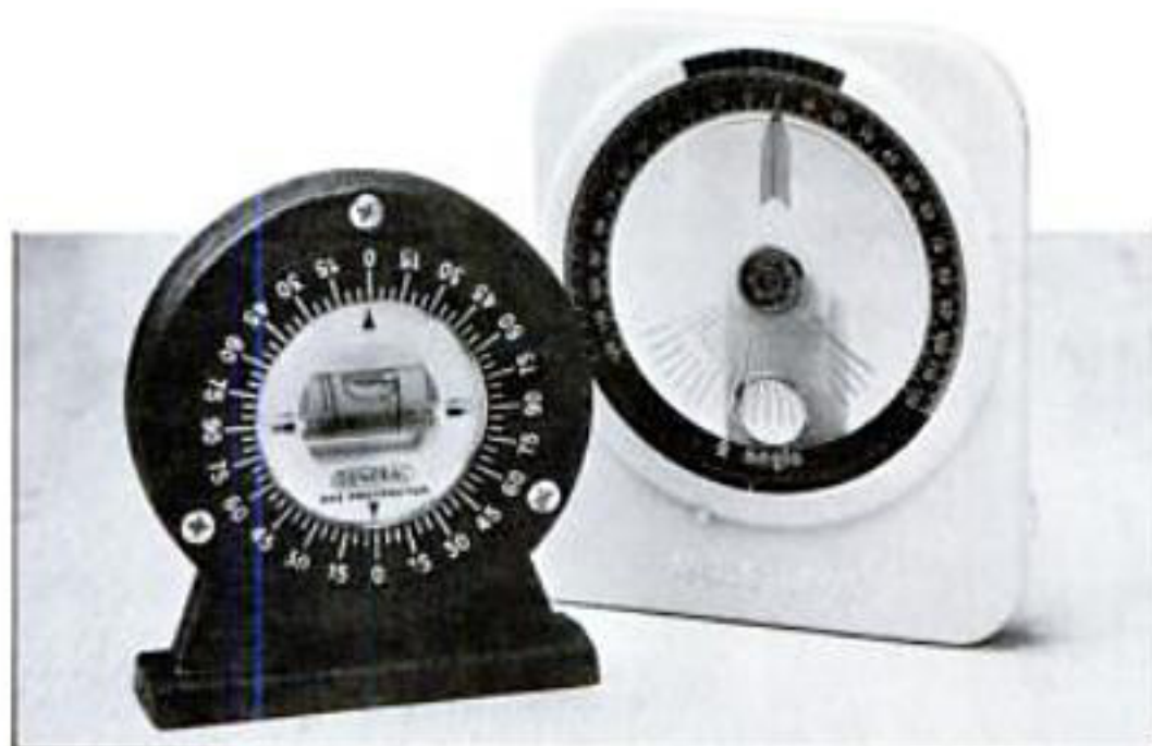
Magnetic angle-finders can help you set the proper bevel angle when you use a honing guide.
