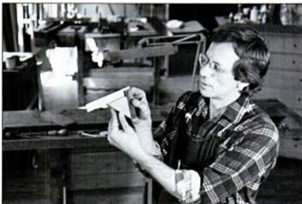
To test the 45° miter-gauge stop, make an angled crosscut, flip the piece, and make a second cut. The two 45° add up to 90°, and you can check the setting with a square. Any error will show up doubled.
