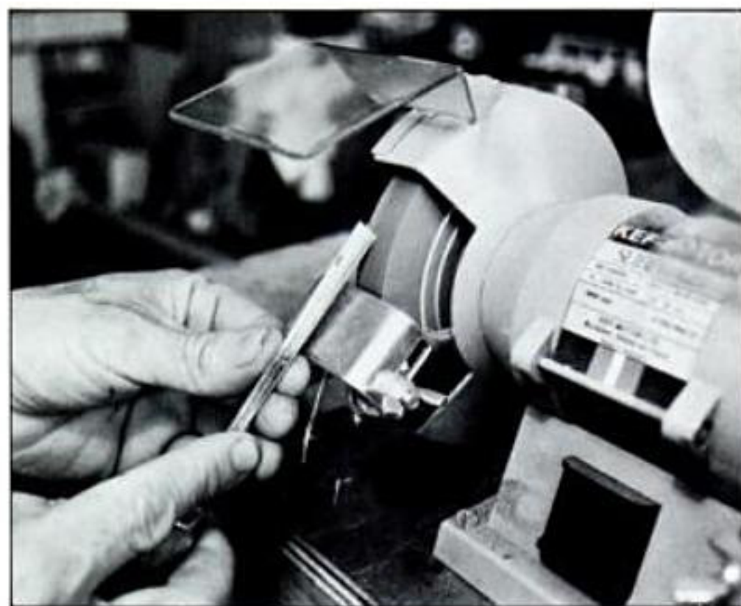
To grind a tool, hold the carving tool with one hand on the handle, the other holding the blade just beneath the rest as shown in the photo.
