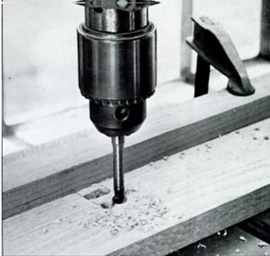
By clamping a fence to the table of your drill press, you'll drill the twin mortises more accurately.
