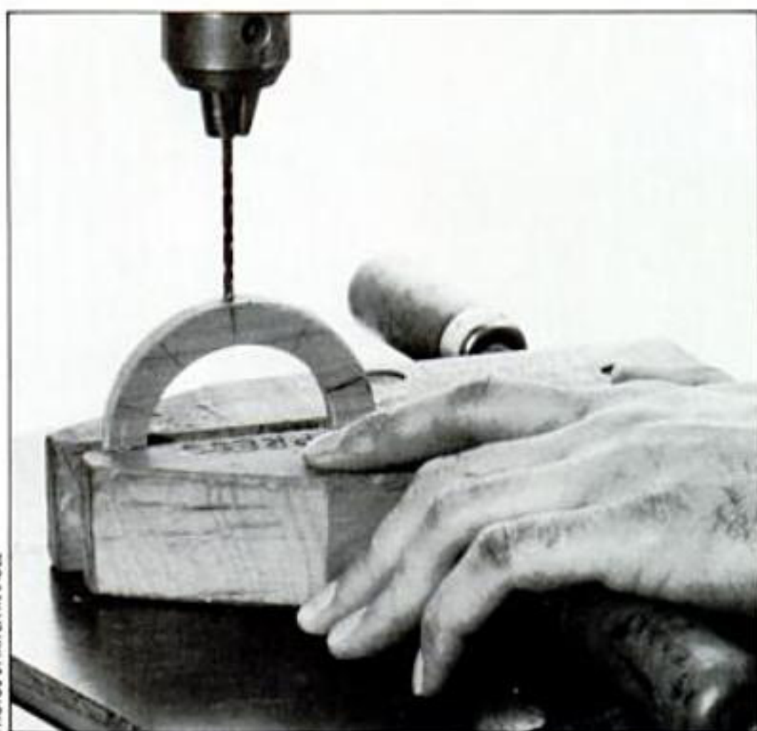
To drill holes for the brass tubes in the spoke-hole guide, hold the guide square to the drill-press table in a wooden hand-screw.
