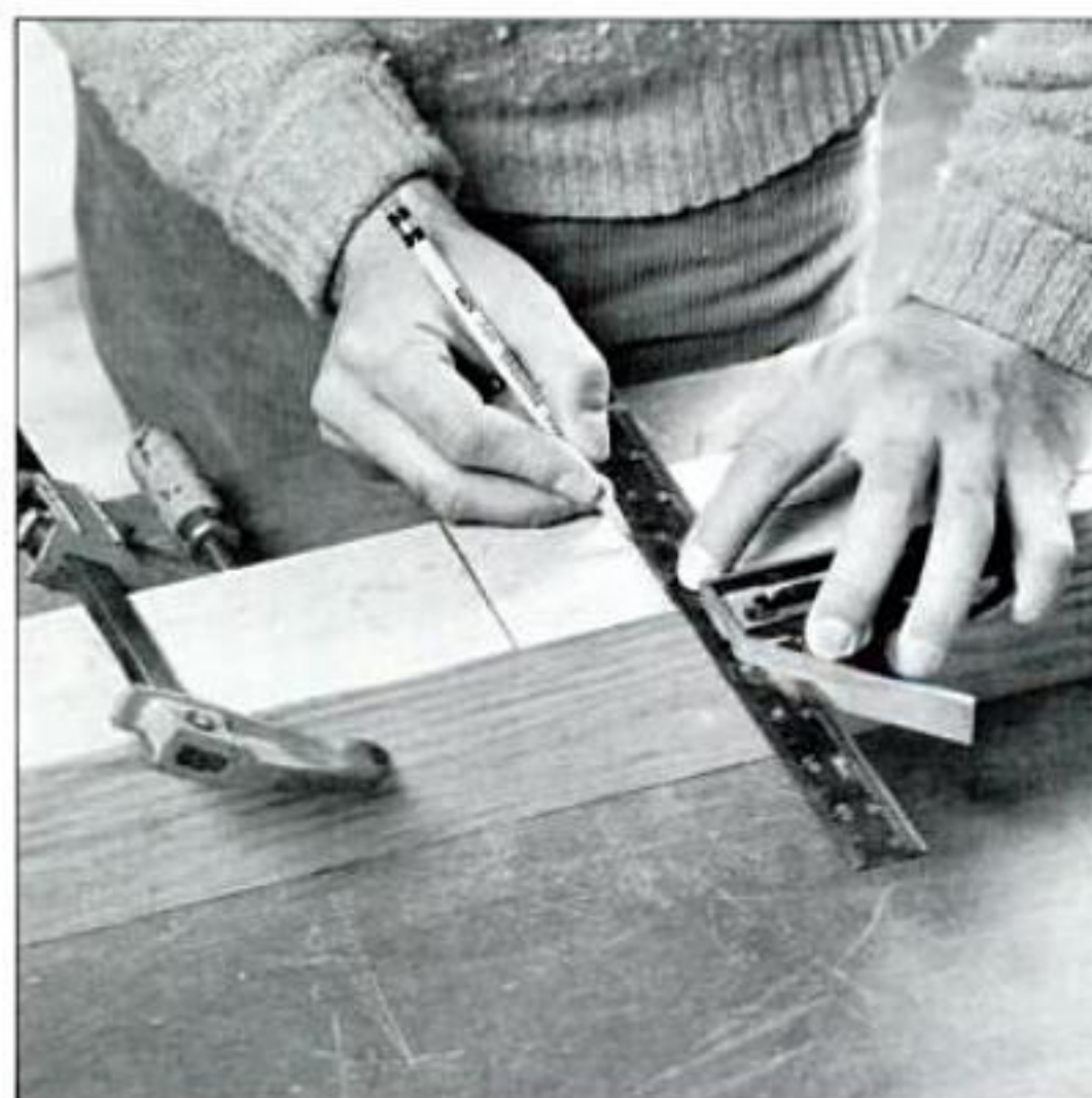
Save time and ensure accuracy by laying out the rail mortises on all four stiles simultaneously.
