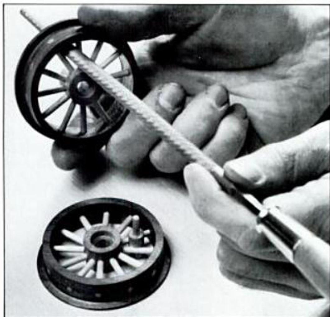
Attach the connecting rods to locomotive driving wheels with a pin made from two dowels. File two spokes to accept the pin and glue the pin between the spokes.
