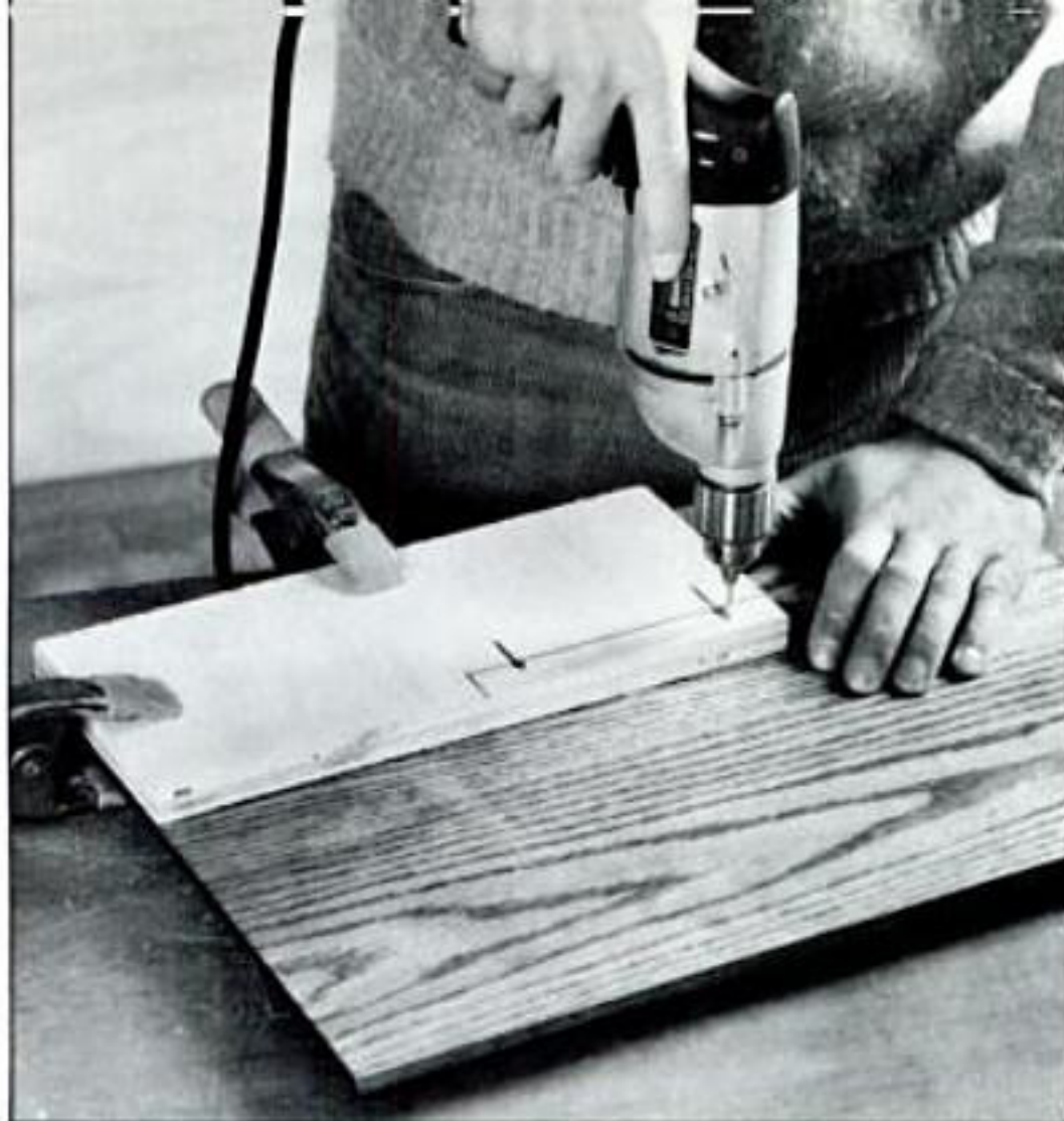
This very basic jig will ensure that the handles are uniformly positioned on the drawer fronts.
