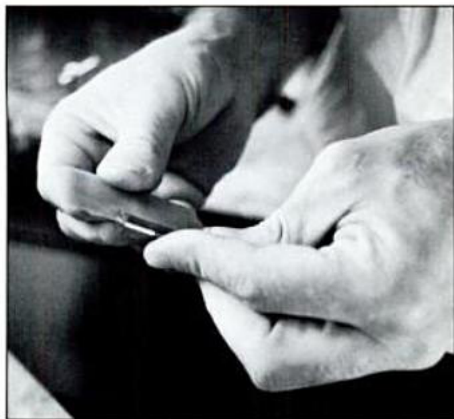
For small tools, hold the tool in one hand and draw the slip stone over the inside with the other.
