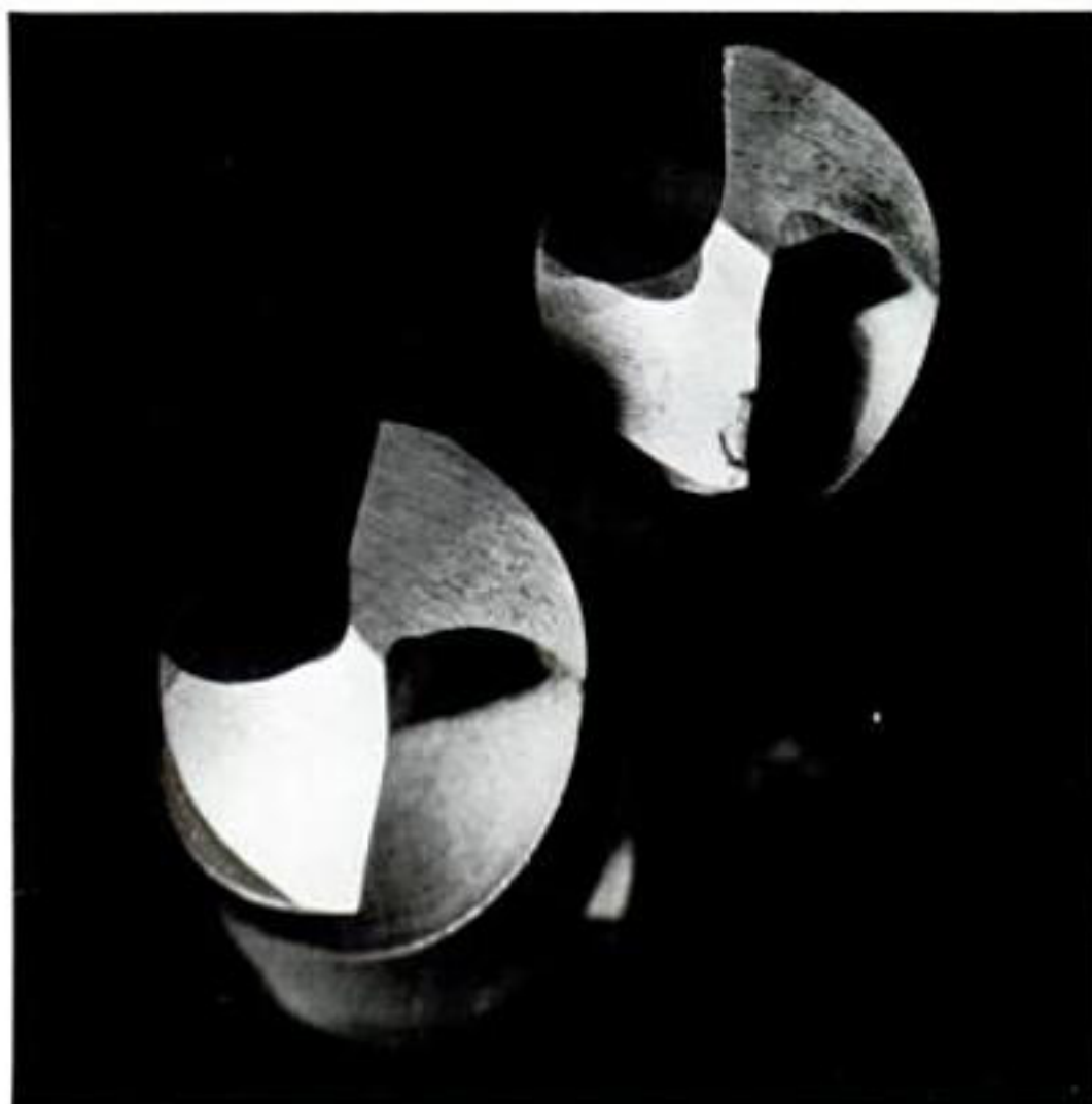
Grinding the damaged lips on the bit in the rear will produce a sharp bit like the one in the foreground.
