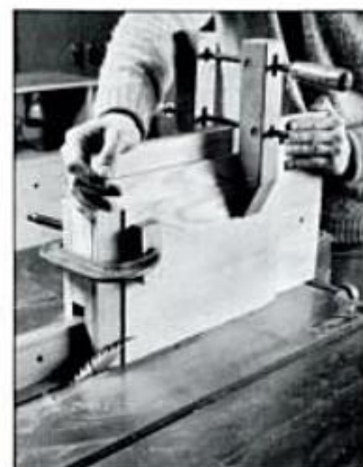
Clamp your panel to the panel-raising jig and push it slowly over the saw. Cut the two end-grain edges first, then the long-grain edges, and, presto, you've raised the panel.
