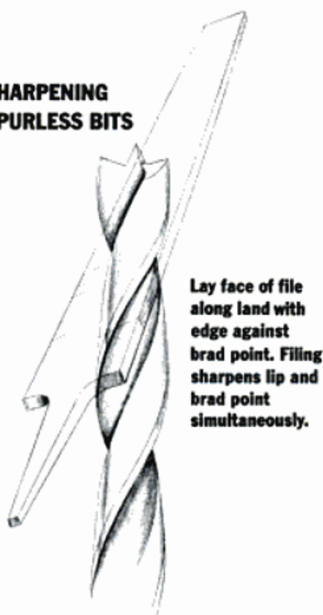
FIG. 3: SHARPENING BRAD-POINT BITS
