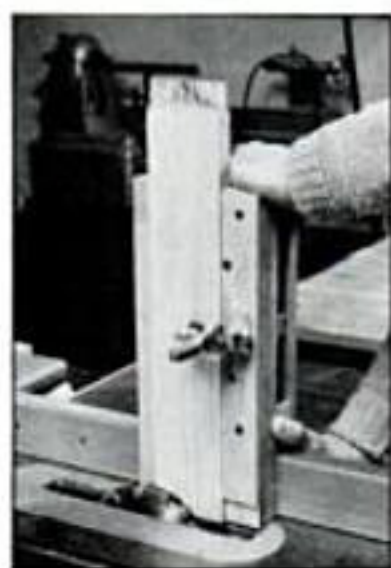
A tenoning jig will make the task of cutting tenons on the tablesaw simple and safe.
