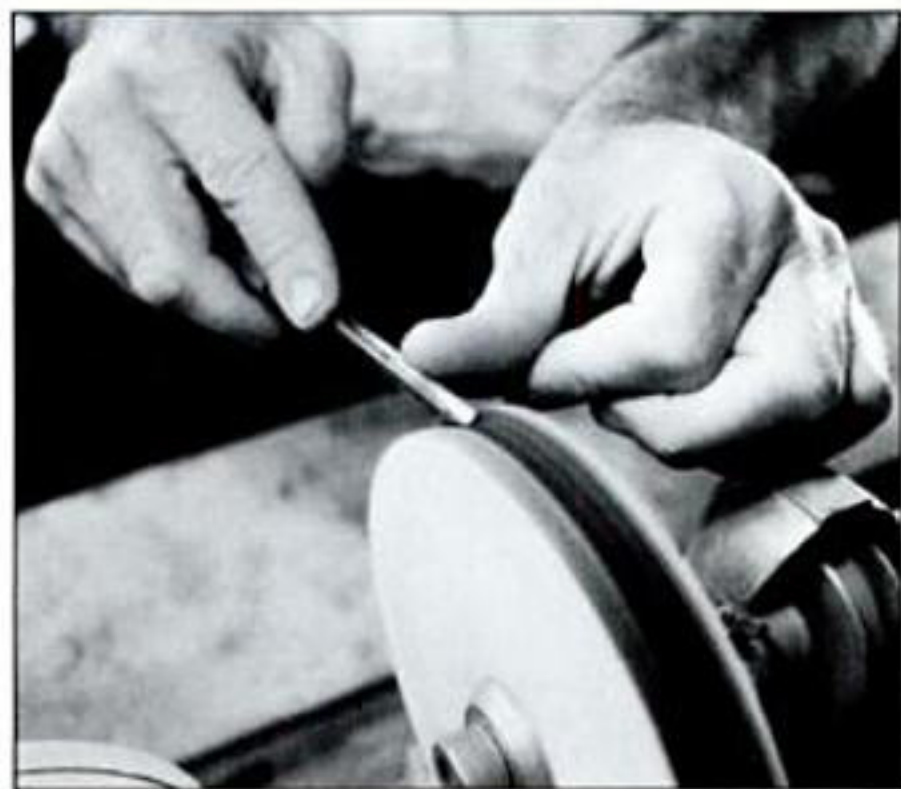
Buffing is an alternative to stropping. A hard-felt wheel charged with an abrasive compound produces a keen edge in a minimum of time.
