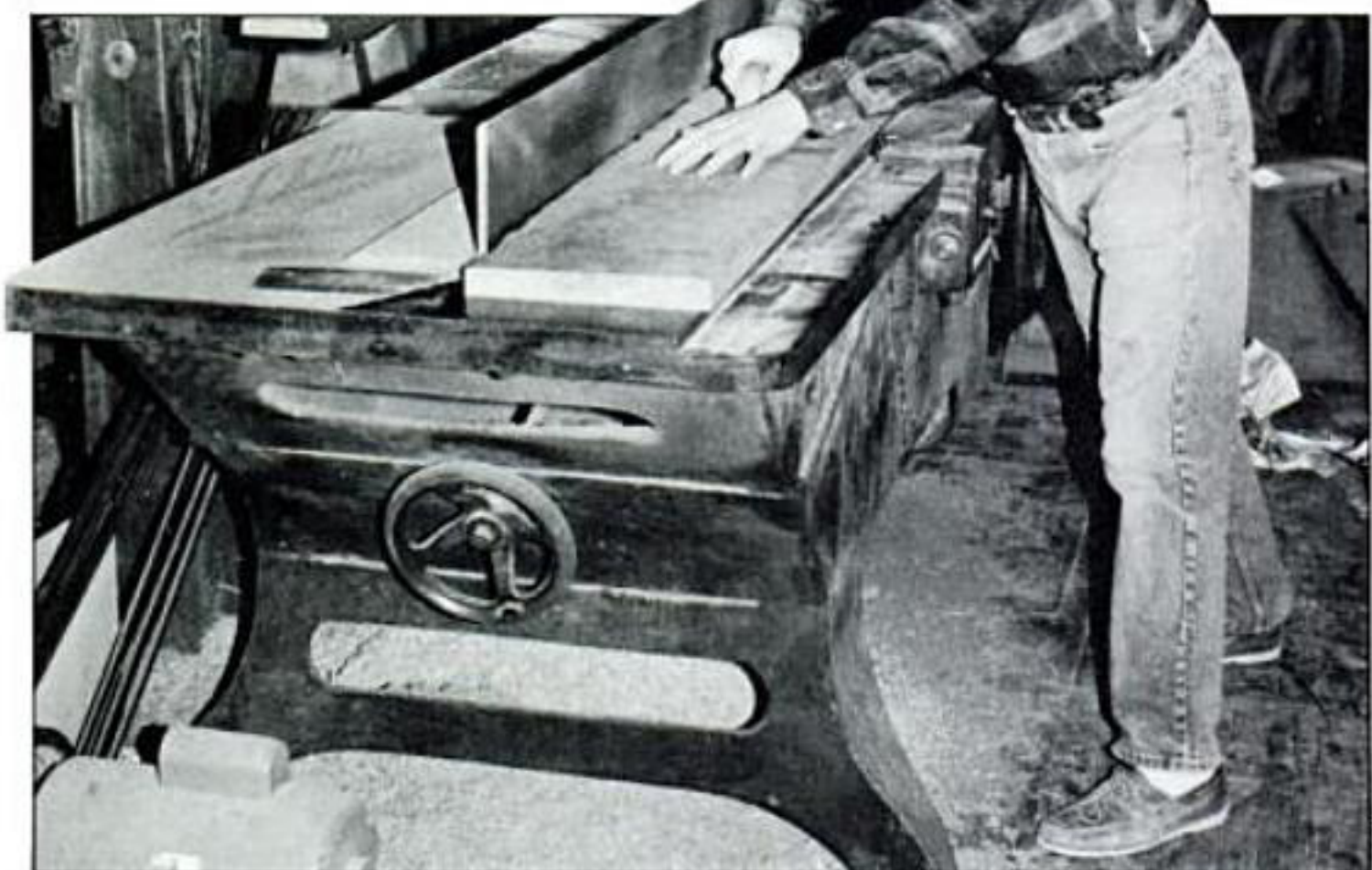
This is the World's Largest Jointer, or so we think. It measures 24 in. wide and 86½ in. long. If you know of a bigger one, enter our Big Jointer Contest.
