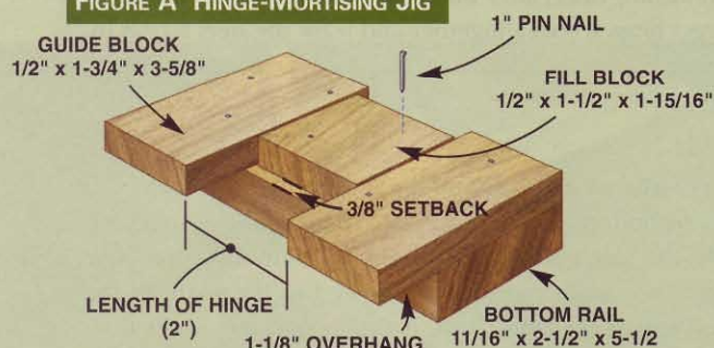
FIGURE A HINGE-MORTISING JIG
