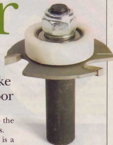
A 1/8-in. slotting cutter is the only bit you need to make this door.
