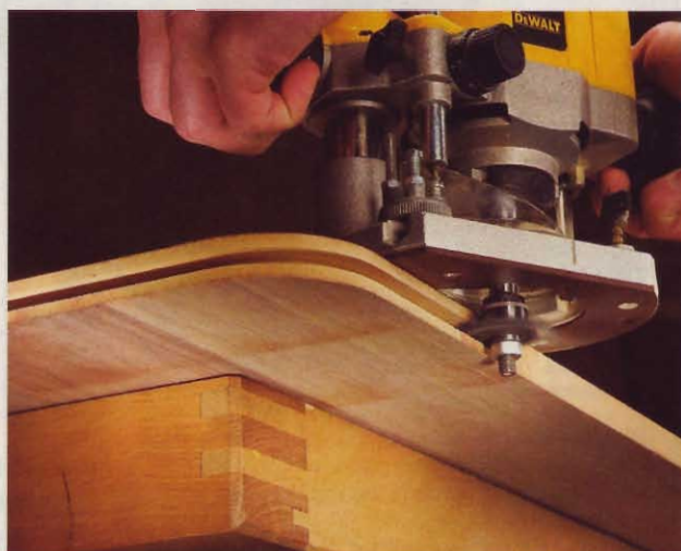
4 Rout the spline slot on the tabletop's edge. Splines align and strengthen the joint between the edging and the tabletop.
