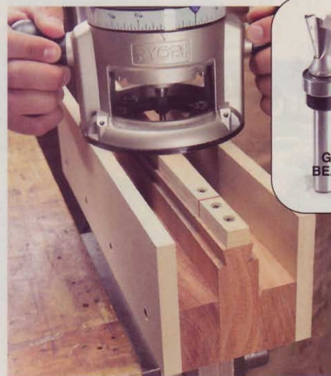
6 Rout the dovetail. Follow the taper template with a dovetail bit that has a bearing above the cutter (see inset).
