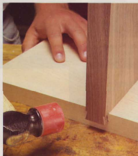
11 Assemble the joint. It will be very loose until you get near the end, because both parts are tapered. You may have to adjust the width of the socket to make it flush and tight with the tail.
