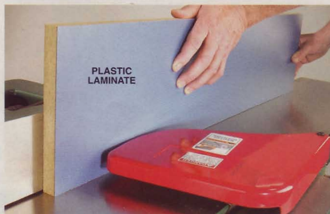
Carbide cutters allow you to joint abrasive manufactured materials, such as plastic laminate, melamine, particleboard and MDF. These materials would destroy the edge on a set of HSS knives.
