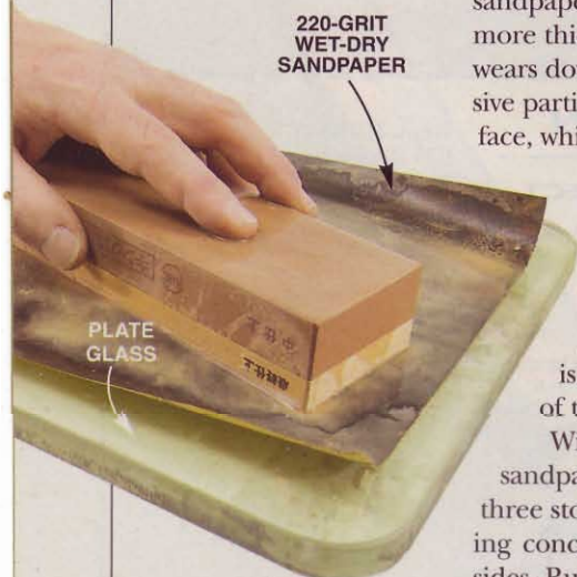
Flatten a combination waterstone with wet-dry sandpaper on glass.
