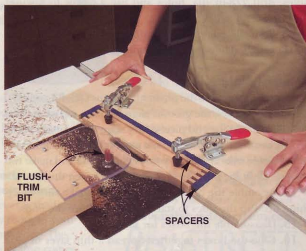
2 Rout the curved ends of all three boxes using the same jig (Fig. B, page 67). The large box's ends exactly fit the opening. Spacers center the ends of the medium and small boxes, so the profiles and handle holes all match.
