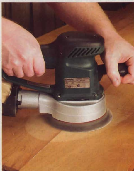
A 6-in. sander works quickly on large areas because its disc has almost 50 percent more sanding surface than a 5-in. sander. All 6-in. sanders have two-handed pistol grips.
