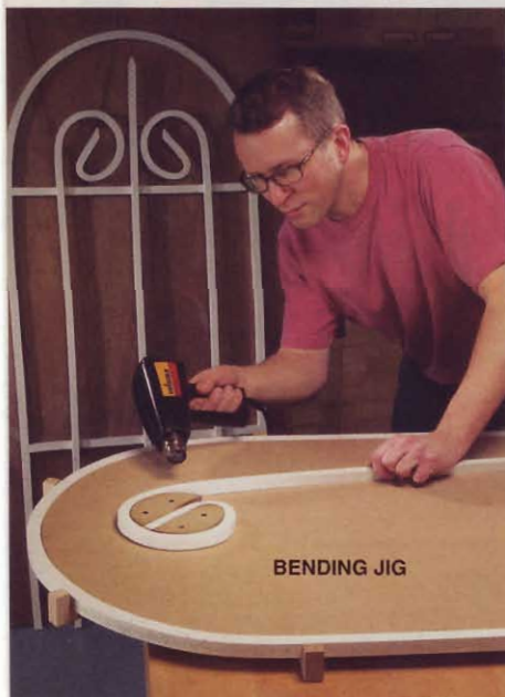
Bending thin strips of plastic lumber is very easy. With a heat gun, a bending jig and a little creativity, you can open up a world of possibilities.
