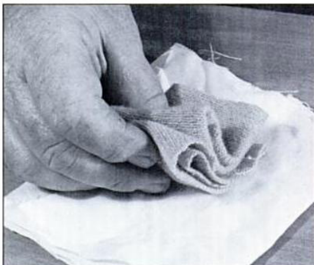
To make a rubbing pad, place a piece of wool from an old sweater inside a linen cover.
