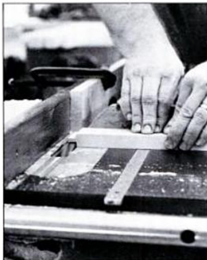
Mill tongues with the dado head raised \frac{1}{4} in. above the table and adjusted for a \frac{1}{2} -in. wide cut. Two passes complete each tongue.
