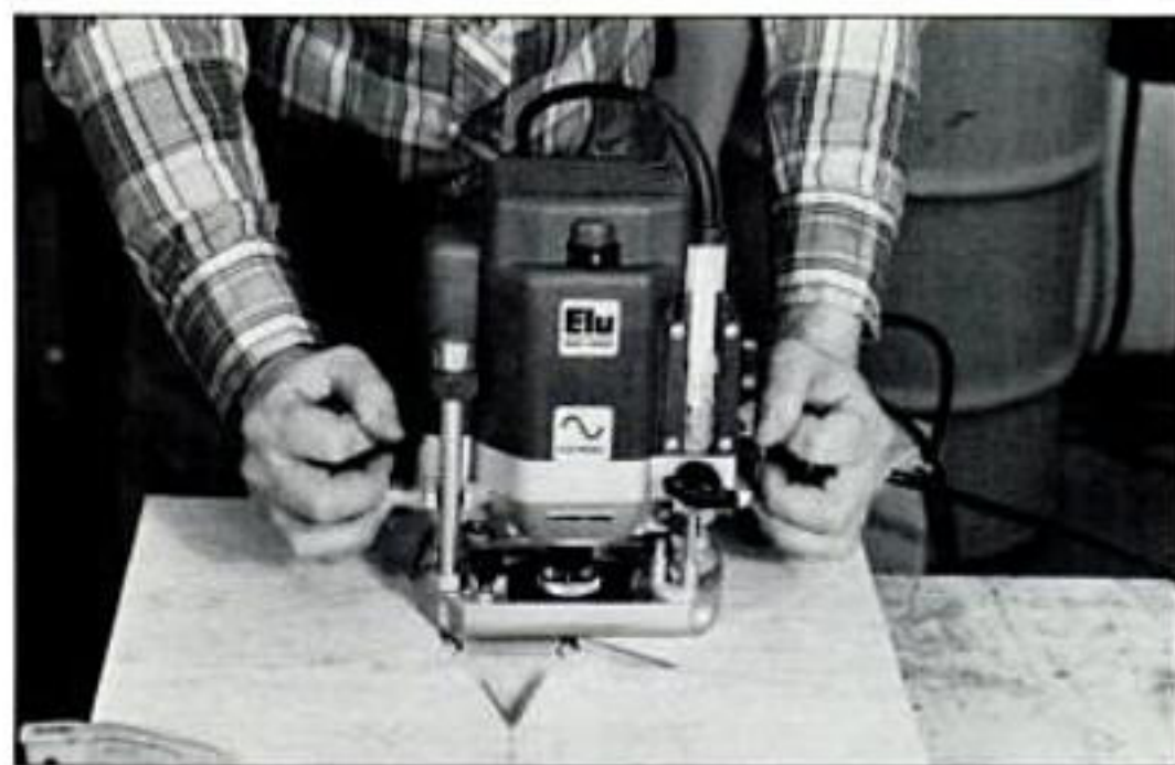
Guide bushings longer than \frac{1}{4} in. require a template made from \frac{3}{8} -in. or \frac{1}{2} -in. material.
