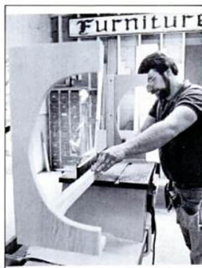
Set up the router table with a \frac{1}{2} -in. cove bit to mill a cove in the top edge of the base.
