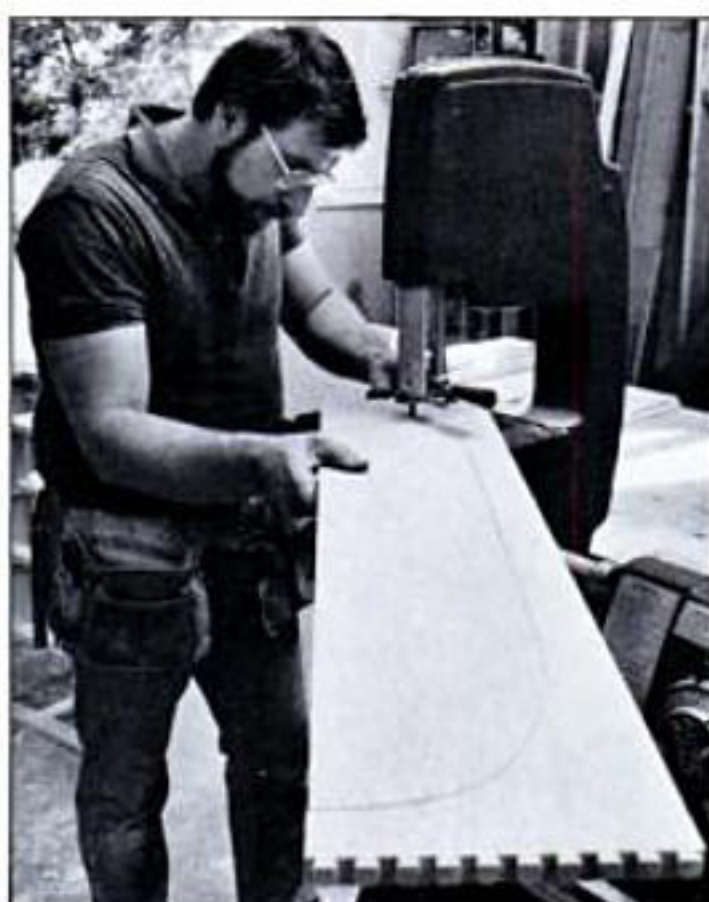
Cut the curved legs out on the bandsaw.
