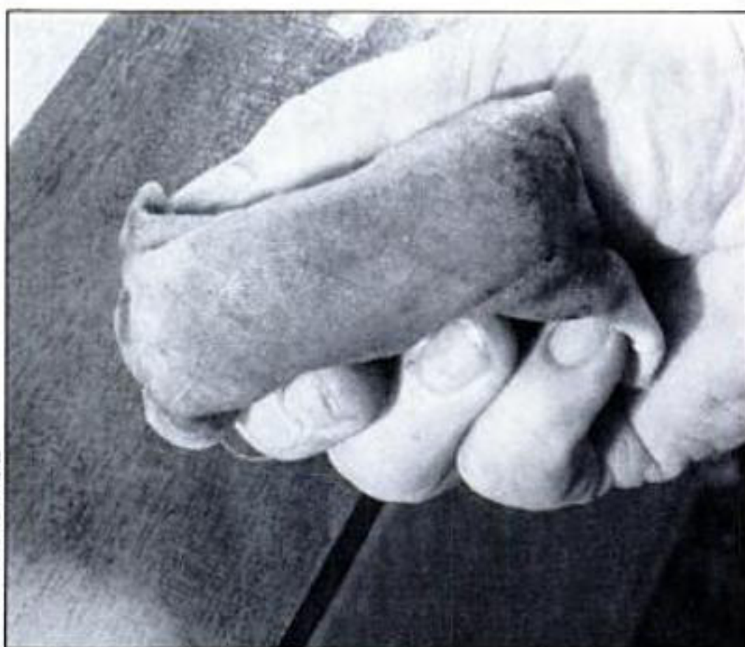
Hold the pad between the thumb and the fingers.
