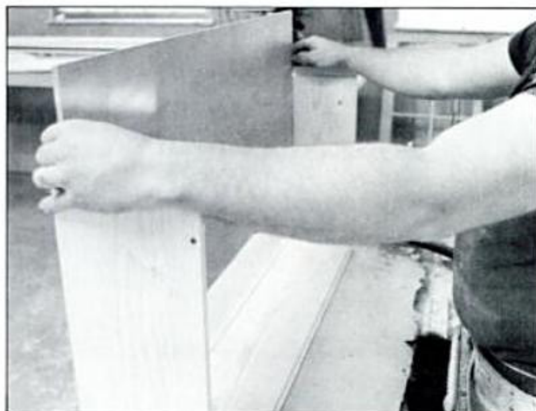
Installing the drawer bottom.
