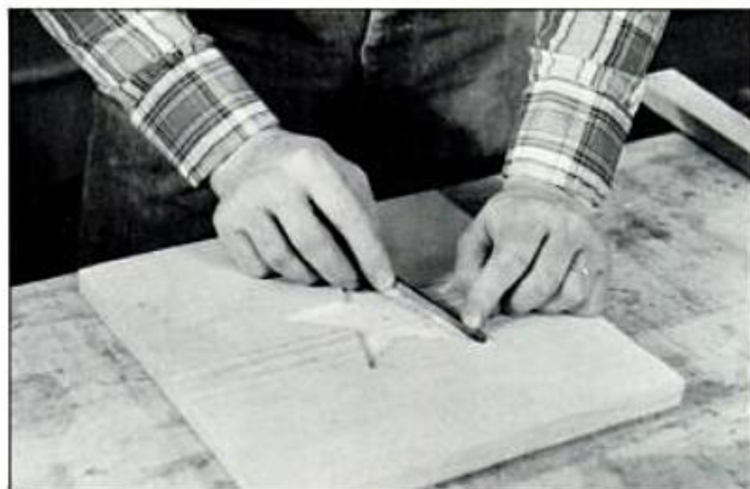
The points of the star-shaped hole are rounded to the radius of the router bit. Trim point with chisel or knife.
