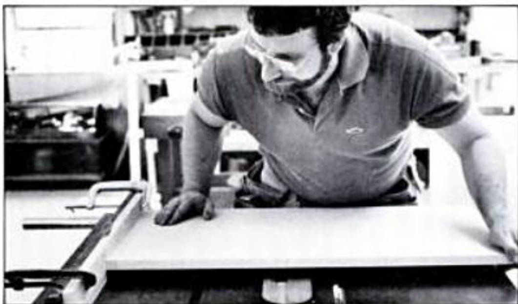
Stopped dados are cut in two steps (photo above and right). First dado the sides on the table saw (above). Use the rip fence as a guide and lower the side over the cutter.
