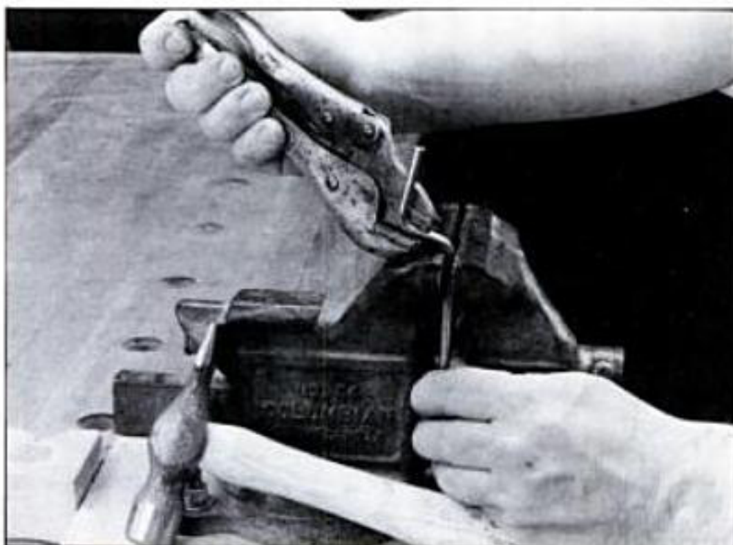
To make the second bend in the crank, grasp the rod with a pair of vise-grip pliers below the first bend. This will keep the first bend from unbending.
