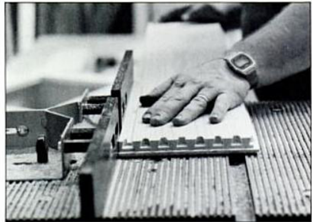
The drawer fronts have been rabbeted along top and side edges and dovetailed for the sides. The final step is to round over the front edges with a 1/4-in. round-over bit in the router table.
