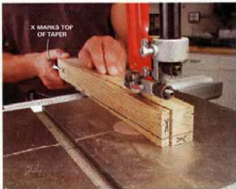
2 Bandsaw two tapers on adjacent sides of each leg. Saw each taper about 1/16 in. oversize. The tapers are subtle, so mark an X at the top of each one to help you keep track of which surface is tapered.
