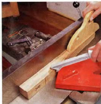
3 Smooth the tapered sides with your jointer. A freehand bandsaw cut can be fairly uneven, so smoothing might take two passes. Feed the legs top-end first. Use a push block and stick to guide the leg.
