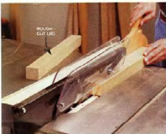
1 Rip thick lumber for the legs to rough size on the table saw. Always use a pushstick when cutting narrow boards. Joint, plane and crosscut the legs to final size.
