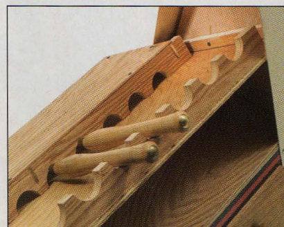
Tools nest in the storage rack.
