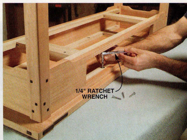
22 Screw the base to the top. Make your own "sideways" screwdriver with a ratchet wrench to get into this tight space. Use a 1/4-in. socket and a screwdriver bit from a cordless drill.
