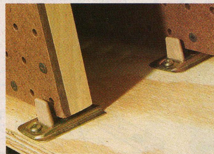
Each door has its own tracking guide. My system uses two sliding-door hardware kits. Each kit contains one guide designed for two doors. I customized them with a hacksaw.
