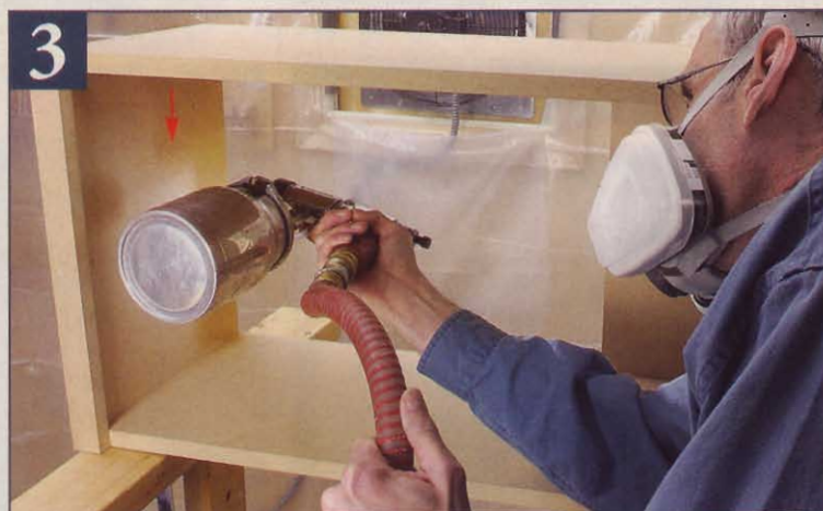
Spray the sides , moving from back to front, away from the overspray.
