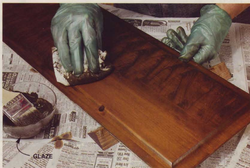
STEP 6 GLAZE ACTS AS A TONER on the sealed surface, resulting in a deep, rich color and a uniform appearance. Just brush it on and wipe it off. Blend uneven areas by varying the amount of glaze you leave on the surface.
