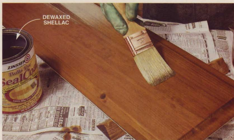
STEP 4 SEAL THE SURFACE with two coats of 2-lb.-cut dewaxed shellac (see Sources, page 92). Sand after each coat with 400-grit paper.
