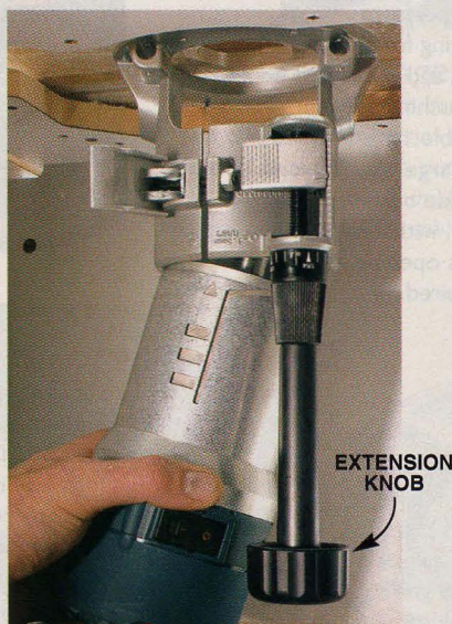
An accessory fixed base ($60) is designed for router-table use, with extra-long screws and an extension knob for easier adjustments to cutting depth.
