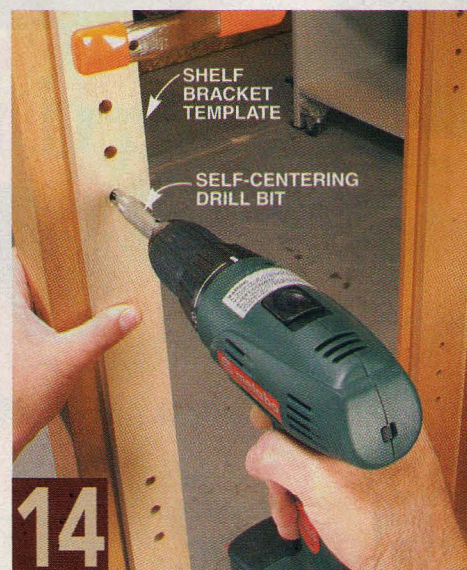
14 Drill the holes for shelf pins. Using a shop-made template and a self-centering drill bit makes this simple and accurate. Align the template with the inside edge of the side stiles.
