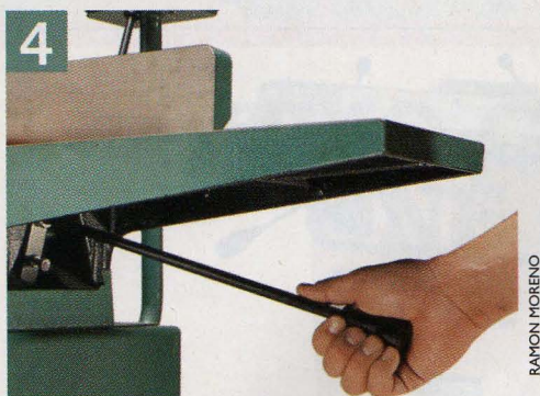
Lever-style table adjusters provide quick, easy adjustment control.
