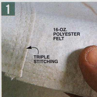
Polyester felt filter bags do a far better job of trapping the small stuff (less than 10 microns) than woven cloth. All bags should be constructed with triple-stitched seams to prevent dust from leaking out.
