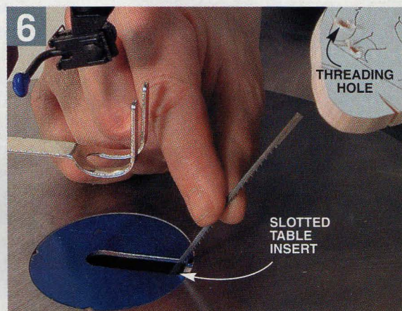
Slotted table inserts allow the blade to tip far enough forward so you can thread the blade through the workpiece.
