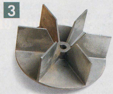
Aluminum or plastic impellers won't produce sparks that can lead to fires from accidentally ingested metal. But they are less durable than steel impellers.
