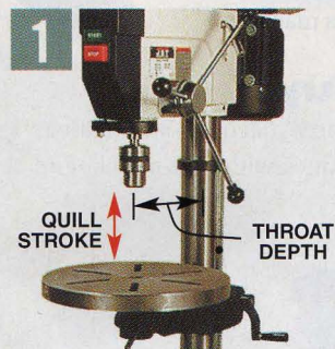
Throat depth and quill stroke determine how far in and how deep you can drill.
