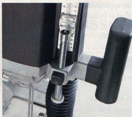
Depth-of-cut indicators, like on this Freud FT2000E, should be easy to read.
