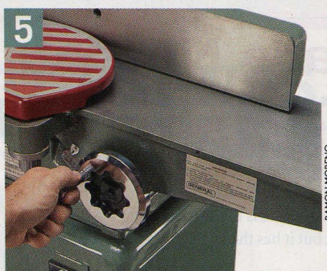
Wheel-style table adjusters provide precise adjustment control. Front-mounted wheel adjusters are more convenient than the under-the-table style.
