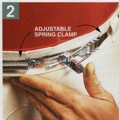
Adjustable spring clamps are best. They make a tight seal and are easy to get on and off.
