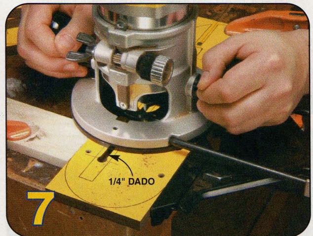
ROUT CLEARANCE DADOES using an edge guide. Center the bit on the guideline.
