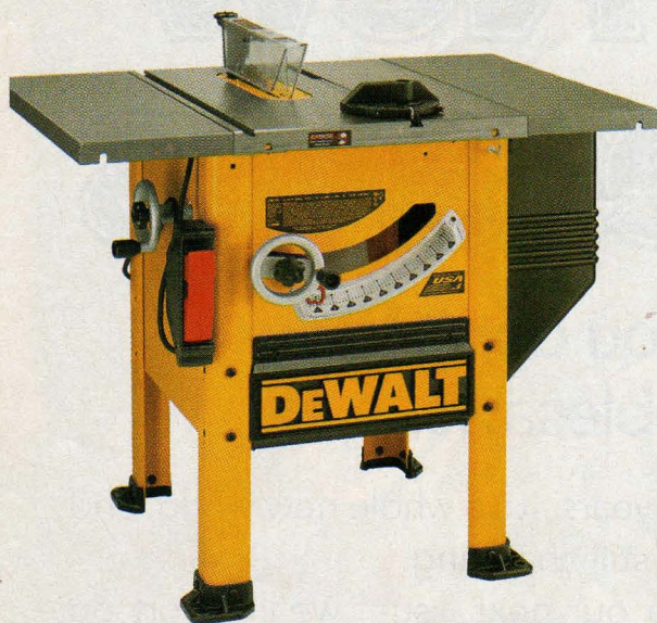
The DeWalt DW746X looks like a contractor's saw, but its motor is tucked inside, like a cabinet saw.
