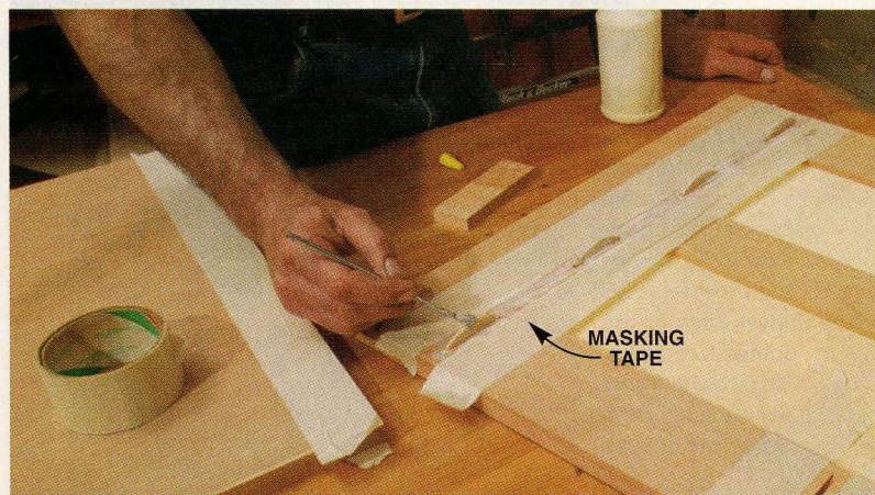
Photo 16 APPLY GLUE in the biscuit slots. White glue gives you slightly more working time, which is convenient for a complicated glue-up like this. The tape makes it easier to remove squeezed-out glue. It's not really necessary on the lower cabinets, but it's useful on the uppers.
