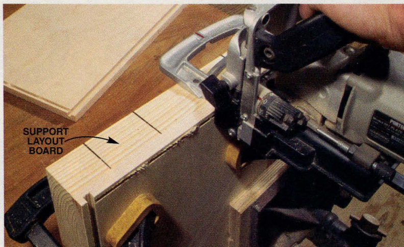
Photo 1 CUT BISCUIT SLOTS for drawers, using a piece of scrap as a support/layout board. With it, you can transfer slot locations to each part of each drawer accurately. Clamped to the drawer side, it also helps support the fence of the plate joiner.
