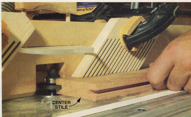
Photo 7 CUT GROOVES in the rails and stiles to house the plywood panels. The center stile (shown) gets grooves on both sides, the others on just the inside edge. Keep the good (outside) face down, and use featherboards and a push stick.
