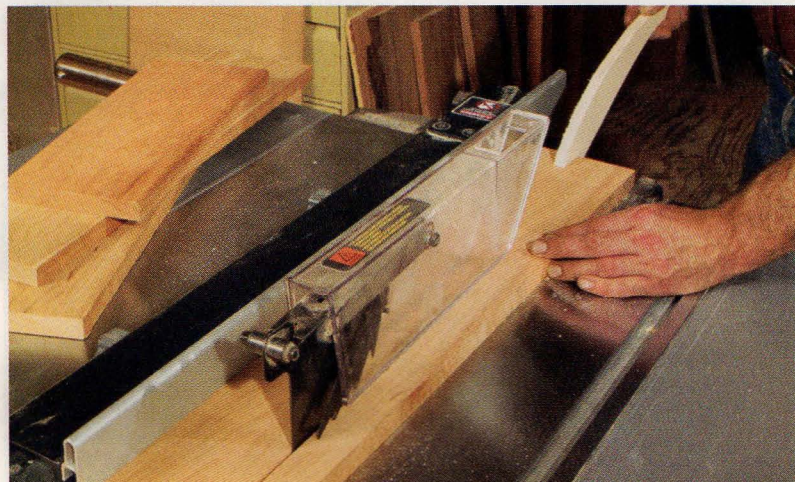
Photo 5 CUT RAILS AND STILES from solid wood, keeping the grain as straight as possible. Cut the center stiles to length later, after marking them against the partially assembled frame.
