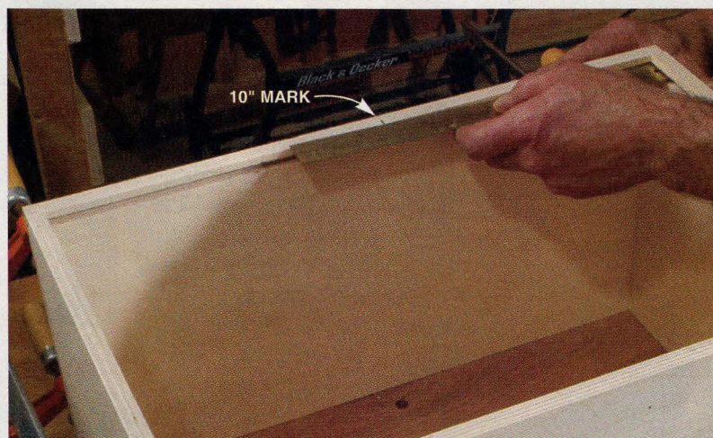
Photo 2 MEASURE GROOVE TO GROOVE to ensure the drawer bottom is the right size. Mark a convenient distance from the bottom of one groove (in this case, 10 in.), then measure from the other groove to your mark.
