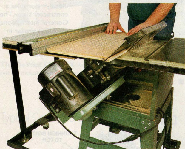
Left-tilt saws are now available from many manufacturers. They cost no more than right-tilt models. The blade tilts away from the fence on a left-tilt saw.
