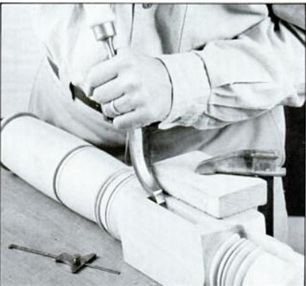
A swan-neck chisel and a depth gauge (on bench) are handy tools for chopping deep mortises.
