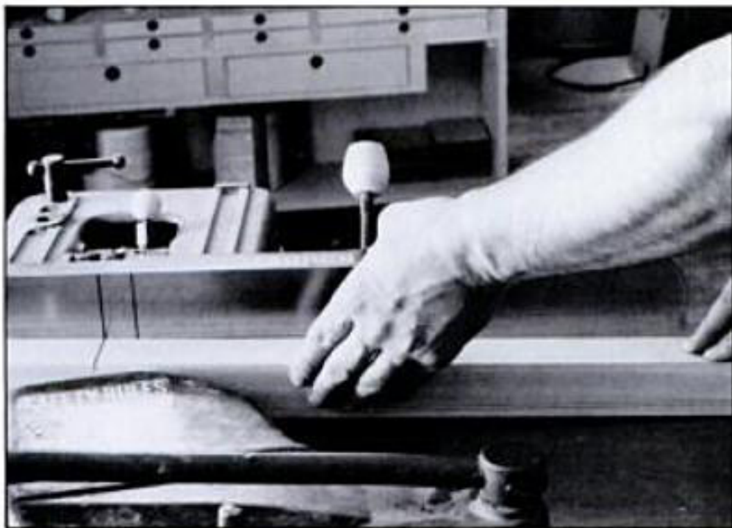
Begin the cut when the reference line on the board is directly over the end of the outfeed table. Mark the fence to indicate this point.
