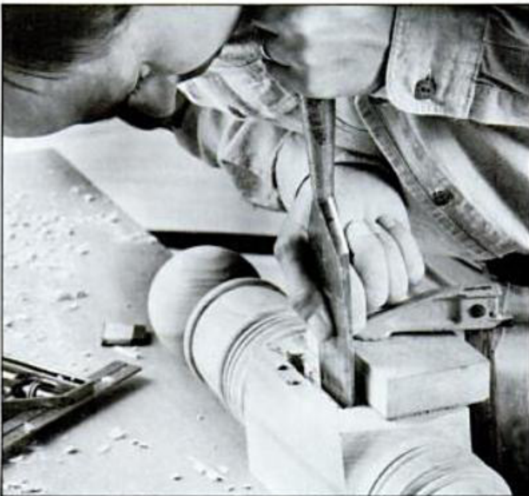
To cut the rail mortises, remove most of the waste with a drill then pare the mortise sides with a chisel.
