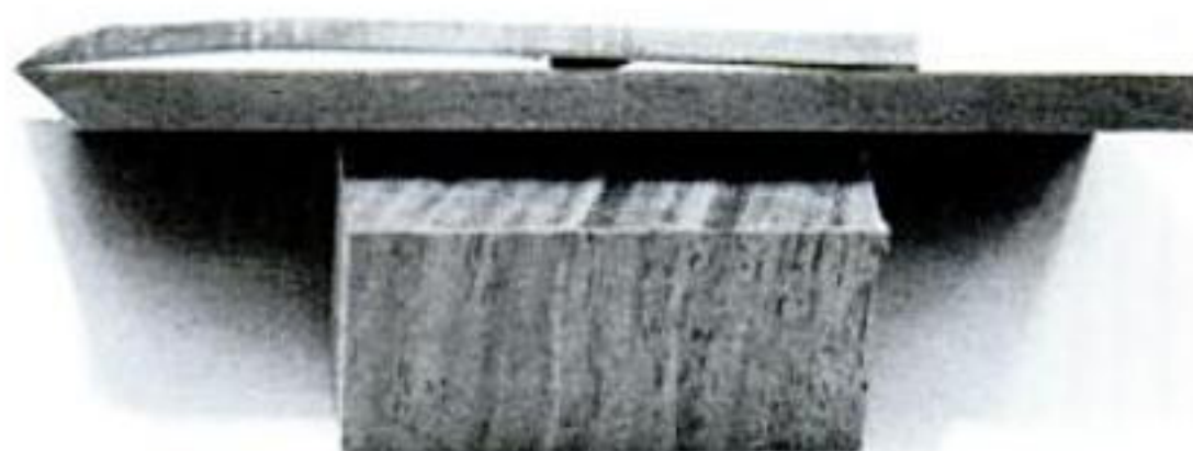
The chip breaker has a gentle curve and a sloping face that allows the shaving to pass up the face of the breaker.
