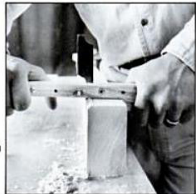
Scrape the bead on the side rails with a shop-made scratchstock.
