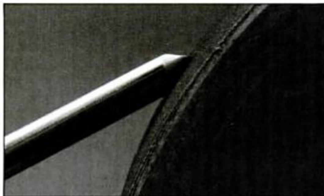
Grinding, the first step in the sharpening process, establishes the shape of the edge and the length of the bevel.
